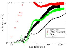
Fig. 11 Reflection vs. log of time for a CLC mixture in a cell with four anchoring situations. The red squares represent a hybrid alignment cell; the black circles represent a rubbed bare glass cell, the green circles represent PVA, and the black line is the PI-2555 alignment layer.
