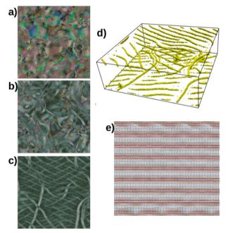
Fig. 5 PW sample for  $K_{33}/K_{22} = 0.067$ . (a)–(c) Calculated textures at t = 0.38 ms, t = 2.78 ms, and t = 496.12 ms, respectively. (d) A mesh of  $\lambda$  lines near the substrates after the CLC structure is formed in the bulk. (e) The director configuration corresponding to (e)
