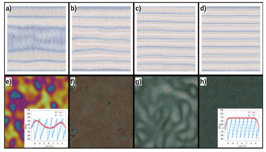
Fig. 6 HS cell for the  $K_{33}/K_{22} = 2.0$  case. (a) –(d) The director field, and (e) –(h) the corresponding calculated textures at t = 0.13 ms, t = 0.21 ms, t = 1.69 ms, and t = 29.3 ms, respectively. The insets of (e) and (h) show the polar and azimuthal angles across the cell at the corresponding times.
