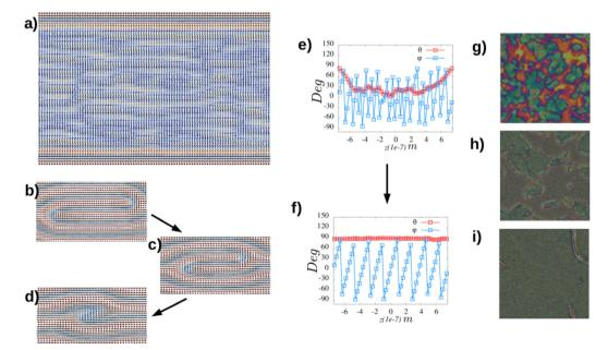
Fig. 3 PS cell for  $K_{33}/K_{22} = 0.067$ . (a) The directors at t = 0.14 ms. Twist grows from the walls and everywhere in the bulk ( $P_t < P_0$ ). (b) –(d) The evolution of dislocation defects. (e) and (f) The polar and azimuthal angles across the cell for t = 0.07 ms and t = 9.66 ms, respectively. (g)—(i) The calculated texture at t = 0.21 ms, t = 1.69 ms and t = 9.66 ms.
