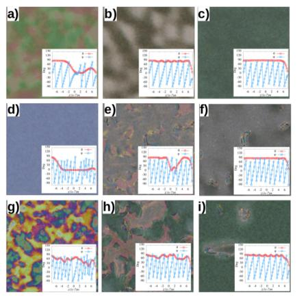
Fig. 9 Calculated textures for the Hyb cell. (a) –(c) The  $K_{33}/K_{22} = 2.0$  case for t = 0.067 ms, t = 0.38 ms, and t = 7.67 ms. (d) –(f) The  $K_{33}/K_{22} = 1.0$  case for t = 0.13 ms, t = 0.92 ms, and t = 9.67. (g)—(i) The  $K_{33}/K_{22} = 0.067$  case for t = 0.067 ms, t = 0.92 ms, and t = 9.67 ms. The insets in all figures show the corresponding polar and azimuthal angles across the cell.
