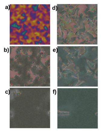
Fig. 7 (a)–(c) The calculated textures for the HS cell for  $K_{33}/K_{22} = 1.0$ , and (d)–(f) the calculated textures for the HS cell for  $K_{33}/K_{22} = 0.067$ . (a) and (d) are calculated for t = 0.57 ms, (b) and (e) for t = 1.69 ms and (c) and (f) for t = 29.3 ms
