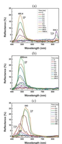
Fig. 10 Reflection spectra during the transition from homeotropic to planar. (a) The case for  $K_{33} = 1.71K_{22}$ , (b) the case for  $K_{33} = 1.0K_{22}$  and (c) the case for  $K_{33} = 0.89K_{22}$ . Figure reproduced from ref. 34.
