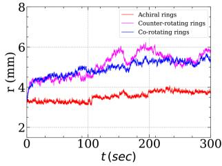
Fig. 8 Time evolution of the distance between two rings at  $\phi$  = 0.775 with an initial separation of  $r_0 = 3.0$  mm for pairs of co-rotating chiral rings, counter-rotating chiral rings, and achiral rings. The distance between achiral rings remains nearly constant, indicating the absence of significant interactions between them.
