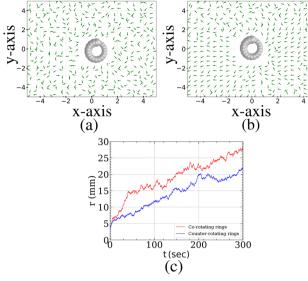
Fig. 7 (a) and (b) The velocity field around a clockwise-spinning ring at  $\Gamma$  = 7 and  $\Gamma$  = 9, respectively. (c) Inter-ring separation as a function of time for co-rotating and counter-rotating rings at  $\Gamma$  = 9. Here,  $\phi$  = 0.775.
