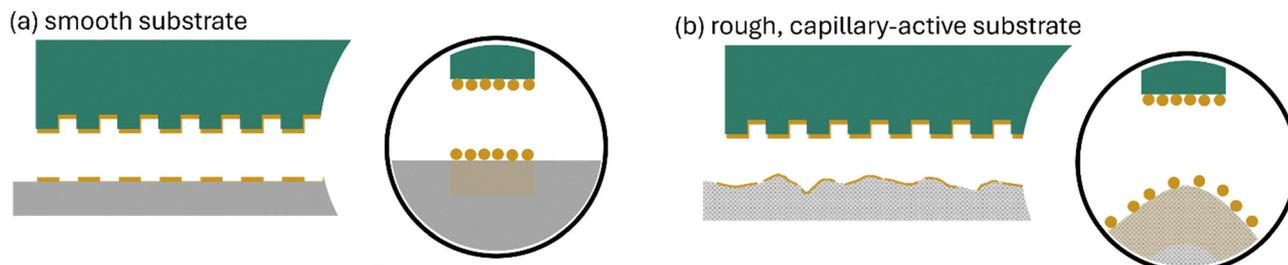
Fig. 21 Microcontact printing on different surfaces. (a) On a smooth surface, a high printing precision can be obtained. (b) On a rough, capillary-active surface, ink smearing occurs, which reduces the printing precision.
