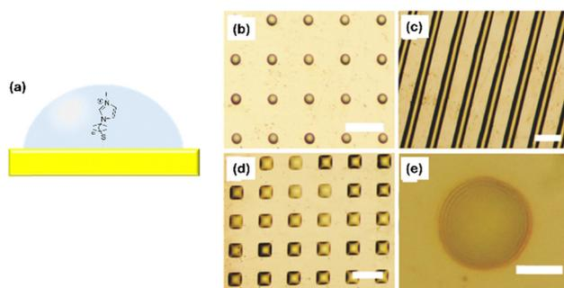
**Fig. 2** Printing of ionic liquids for the deposition of microscale droplets. (a) Chemical structure of the ionic liquid printed on a gold surface. (b)–(e) Different printed patterns. The scale bars are (b) 50  $\mu$ m, (c) 100  $\mu$ m, (d) 50  $\mu$ m, and (e) 10  $\mu$ m. Reproduced with permission.<sup>29</sup> Copyright 2016, the American Chemical Society.
