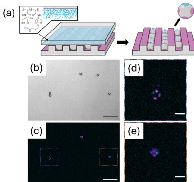
**Fig. 17** Patchy particles fabricated in a confined environment. (a) Schematic representation. (b) Transmission light microscopy image of the particles. (c) Fluorescence microscopy image. (d) and (e) Zoom-in views of the particles. Scale bars: (b) and (c) 25 μm. (d) and (e) 5 μm. Reproduced with permission.<sup>134</sup> Copyright 2025, Wiley.
