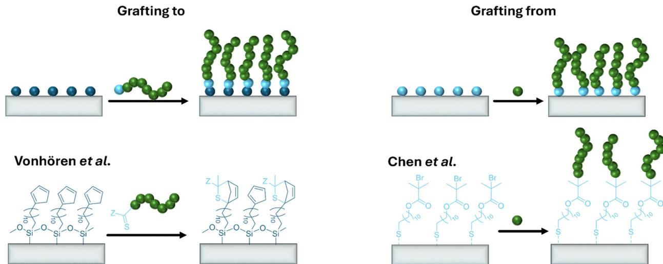
Fig. 6 Grafting to vs. grafting from-approach. The approach from Vönhören *et al.* is illustrative for the grafting to,<sup>75</sup> by Chen *et al.* for the grafting from-approach.<sup>76</sup>
