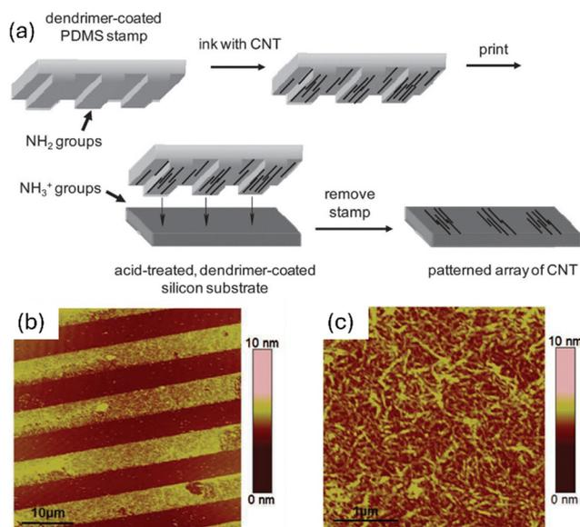
Fig. 20 Printing of carbon nanotubes (CNTs). (a) Schematic overview. (b) Printing pattern. (c) Zoom-in view of the printed pattern. Reproduced with permission.<sup>135</sup> Copyright 2012, Wiley.
