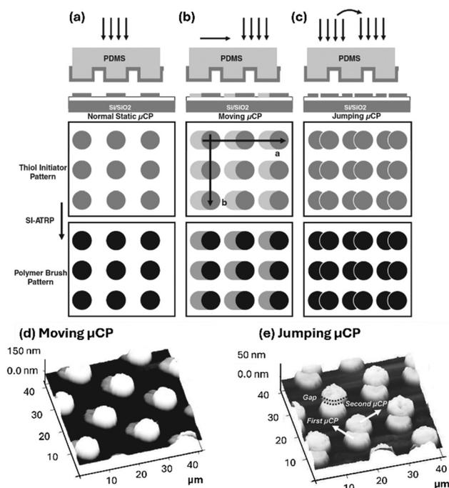
Fig. 7 Dynamic  $\mu$ CP. (a) In contrast to static  $\mu$ CP, dynamic moving (b) or jumping (c)  $\mu$ CP yields intricate patterns. Grafting polymer brushed from the printing areas yields polymer brush patterns as shown in (d) (for moving  $\mu$ CP) and (e) (for jumping  $\mu$ CP), respectively. Reproduced with permission.<sup>83</sup> Copyright 2011, Wiley.
