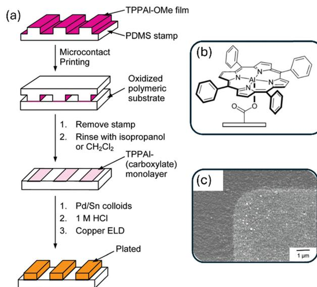
Fig. 19  $\mu$ CP of a copper nanoparticle array using an aluminum porphyrin as an anchor. (a) Overall scheme. (b) Binding of the porphyrin complex serving as an anchor for copper nanoparticle formation. (c) Scanning electron micrograph of the printed pattern. Reproduced with permission.<sup>145</sup> Copyright 2010, the American Chemical Society.
