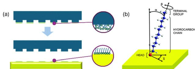
**Fig. 1** Printing of a self-assembling monolayer (SAMs) using an alkylthiol on a gold surface. (a) Schematic overview over the printing process. (b) Binding of the alkylthiol to the surface. Reproduced with permission.<sup>23</sup> Copyright 2010, Royal Society of Chemistry.
