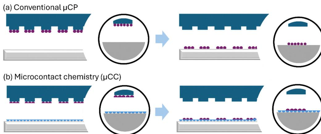
Fig. 4 Conventional microcontact printing ( $\mu$ CP) vs. microcontact chemistry ( $\mu$ CC). (a) In conventional  $\mu$ CP, the ink is transferred from the stamp to the substrate, where it physi- and chemisorbs. (b) In  $\mu$ CC, a reaction partner that is attached to the substrate is reacted with the ink, when the stamp and the substrate contact each other.
