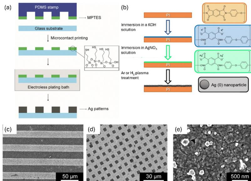
Fig. 18 Printing of AgNPs by using a silver precursor. (a) Schematic representation of the process using a MPTES,<sup>142</sup> and (b) a polyimide polymer.<sup>143</sup> (c) and (d) Printed particle patterns and (e) zoom-in thereof.<sup>142</sup> Reproduced with permission.<sup>142,143</sup> Copyright 2013 and 2014, Elsevier.
