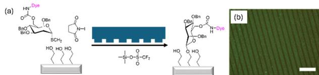
Fig. 5  $\mu\text{CC}$  for binding a carbohydrate (mannose) via glycosylation to a hydroxy-functional surface. (a) Chemical principle. To the substrate, a stamp with the catalytically active species TMSOTf is added. (b) Pattern of mannose formed by  $\mu\text{CC}$ . The scale bar is 50  $\mu\text{m}$ . Reproduced with permission.<sup>72</sup> Copyright 2017, the Royal Society of Chemistry.
