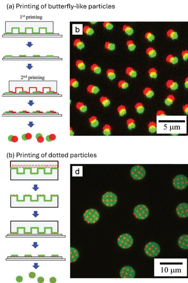
Fig. 14 Printing of anisotropic microparticles created by a layer-by-layer approach. (a) Printing of butterfly-like particles. (b) Printing of dotted particles. Reproduced with permission.<sup>126</sup> Copyright 2011, Wiley.
