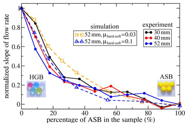
Fig. 4 The slope of flow rate curve obtained by linear fitting between  $0.2 < m/m_{\text{total}} < 0.7$  (see the two black dotted lines in Fig. 3) as a function of ASB concentration. The slope is normalized by the slope value obtained for 0% ASB.
