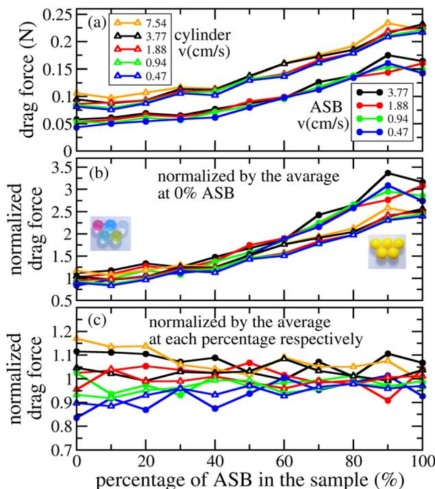
Fig. 7 (a) Drag force on an object (Airsoft bead or vertical cylinder) moved horizontally in the mixture, immersed at a depth of 22 mm. The curves correspond to different velocities  $v$  of the object, the values of  $v$  are indicated in the figure. (b) and (c) Same data as in panel (a) normalized by the average force at 0% ASB (panel b), and normalized by the average force calculated for each concentration (panel c).
