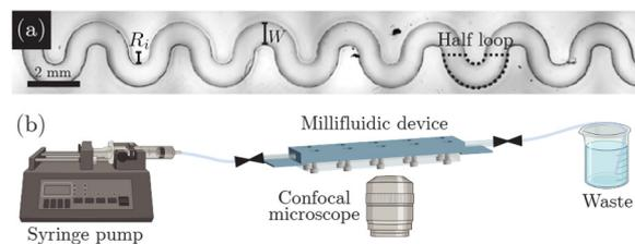
Fig. 2 Serpentine channel geometry and experimental setup. (a) Bright-field optical image of the serpentine channel device comprised of 19 semi-circular half-loops with inner radius  $R_i$  and channel width  $W$ . (b) Schematic of experimental setup for flow visualization.
