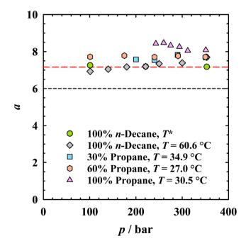
Fig. 7 Geometric prefactor  $a = 2d_{TS}S/V$  as a function of pressure for the studied symmetric bicontinuous microemulsions. The black short dashes denote a = 6, as theoretically predicted by de Gennes and Taupin.<sup>68</sup> Red long dashes denote a = 7.16, as experimentally determined by Sottmann et al. 36 The 1 bar measurement is omitted due to a non-comparable impact of multiple scattering in the 1 mm Hellma cuvette
