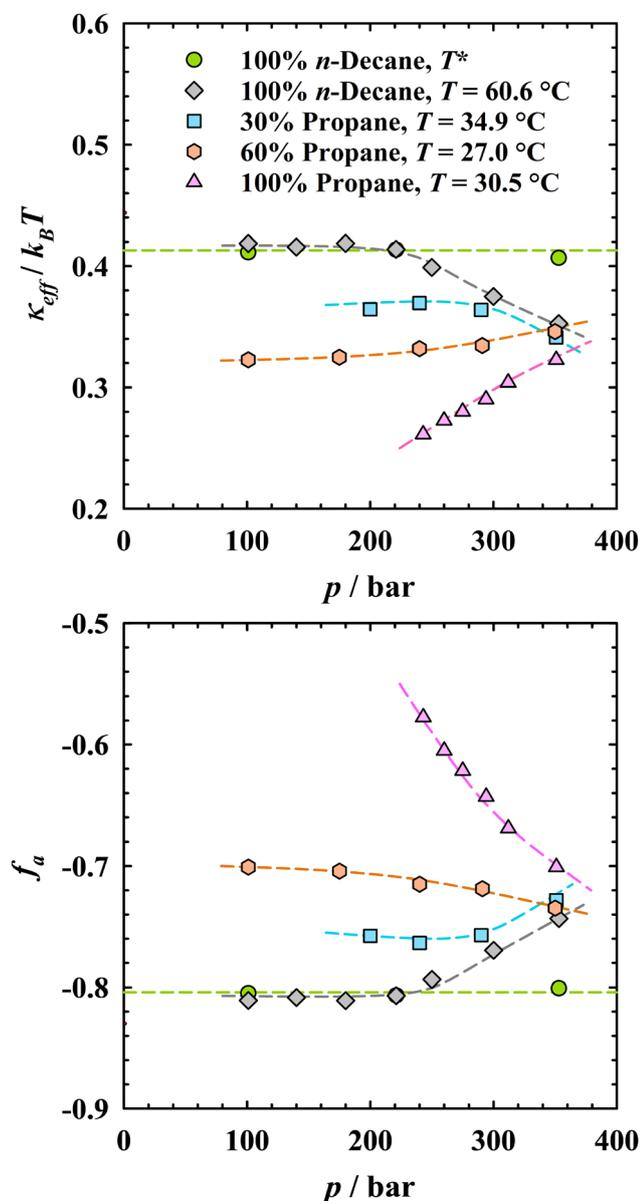
Fig. 8 Pressure dependence of effective bending rigidity  $\kappa_{\text{eff}}$  (top) and amphiphilicity factor  $f_a$  (bottom) for the investigated microemulsions. Dashed lines to guide the eye. The 1 bar measurement is omitted due to the lower impact of multiple scattering in the 1 mm Hellma cuvette.
