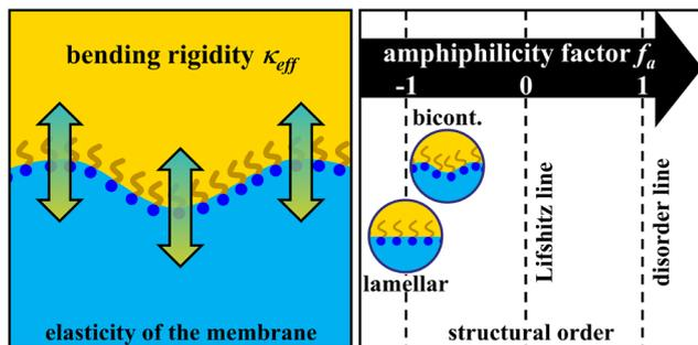
Fig. 1 Left: Schematic illustration of the (effective) bending rigidity  $\kappa_{\text{eff}}$  of the surfactant membrane (amphiphilic film). The higher  $\kappa_{\text{eff}}$ , the stiffer the membrane. Right: Scale of the amphiphilicity factor between  $-1$  and  $1$ . Well-structured microemulsions are located at  $f_a < -0.6$ .<sup>53</sup>
