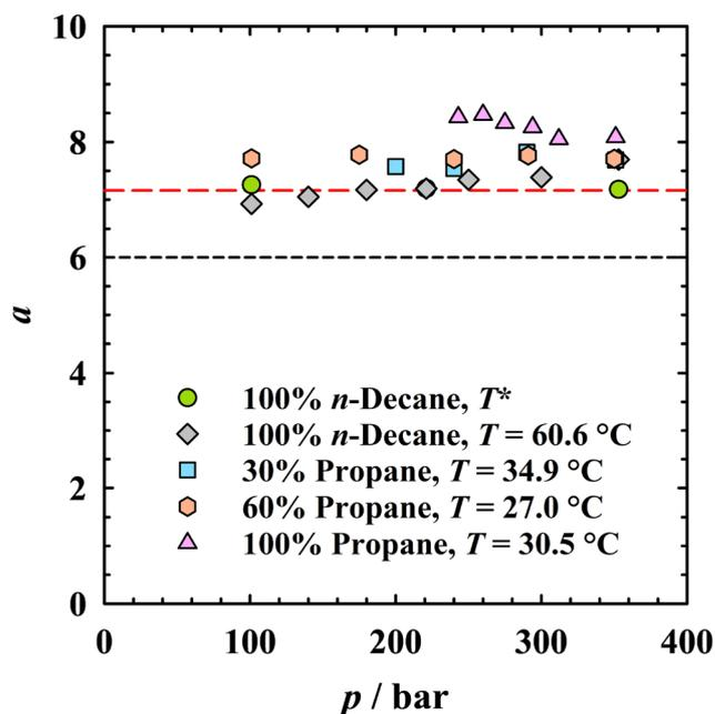
Fig. 7 Geometric prefactor  $a = 2d_{TS}S/V$  as a function of pressure for the studied symmetric bicontinuous microemulsions. The black short dashes denote  $a = 6$ , as theoretically predicted by de Gennes and Taupin.<sup>68</sup> Red long dashes denote  $a = 7.16$ , as experimentally determined by Sottmann *et al.*<sup>36</sup> The 1 bar measurement is omitted due to a non-comparable impact of multiple scattering in the 1 mm Hellma cuvette.
