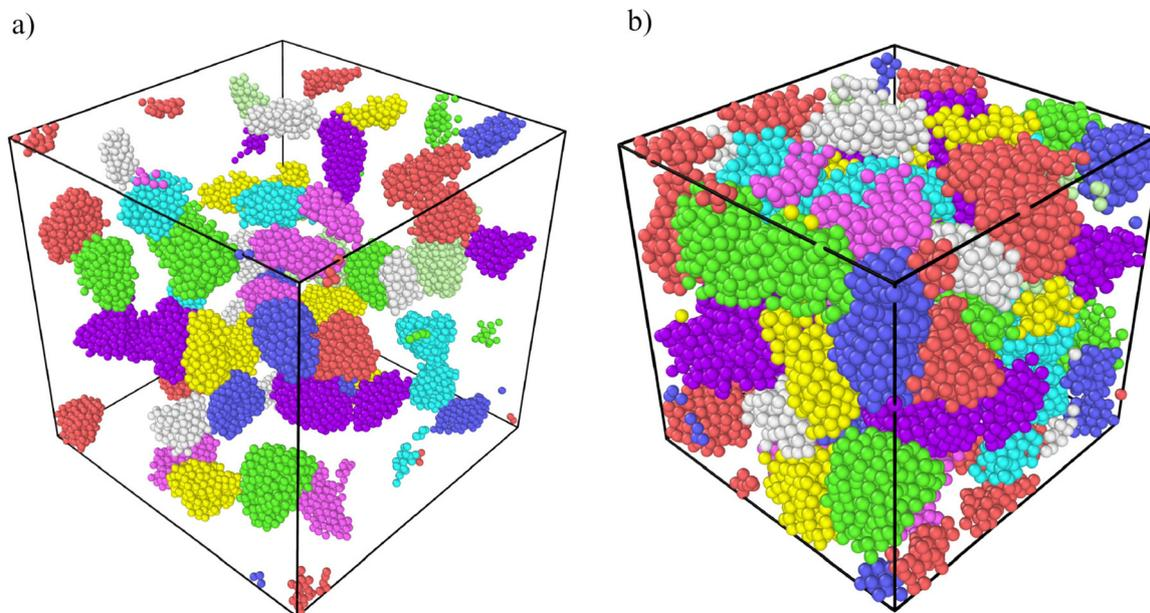
**Fig. 11** (a) The initial arrangement of 50 irregular-shaped BPM grains with  $d_{sp} = 0.100$  for one realization. (b) Final arrangement of irregular-shaped BPM grains for the realization. Individual grains are colored for visibility. The total number of subparticles across all grains in the domain is  $n_{gp}$  and the volume  $V_{gp}$  of the grain packing domain is shown by the black lines of the boundaries. The simulation domain is periodic.
