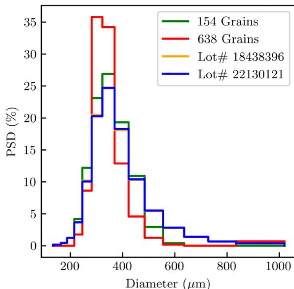
**Fig. 1** Particle size distribution (PSD) of physical silica sand grains: (blue line) particles used in laboratory experiments of jamming packing fraction (Lot# 22130121) (blue line), (orange line) particles imaged by micro-CT and used to generate BPM grain envelopes (Lot# 18438396), (red line) 638 irregular-shaped BPM grains extracted from micro-CT imaging, (green line) reduced set of 154 irregular-shaped grains extracted from micro-CT imaging and used in grain jamming simulations.
