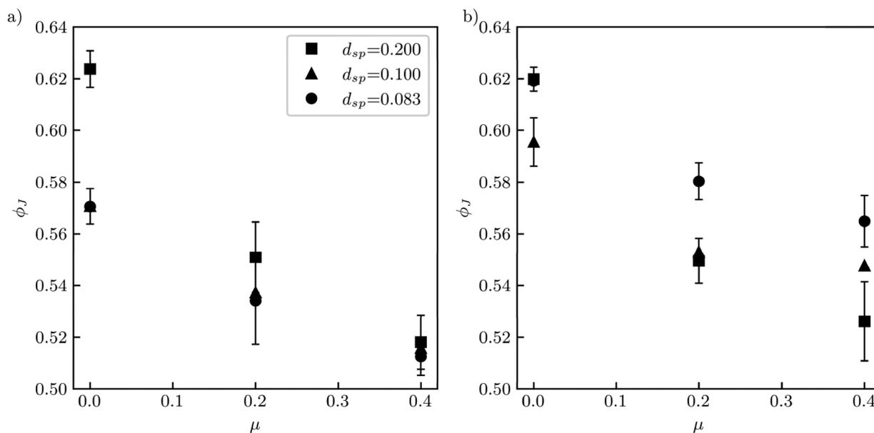
Fig. 13 Plot of jamming packing fraction versus  $\mu$  for (a) regular-shaped (rough) grains and (b) regular-shaped (smooth) grains. Error bars show one standard deviation for  $d_{sp} = 0.083$  and 0.200 with 5 replicates each.
