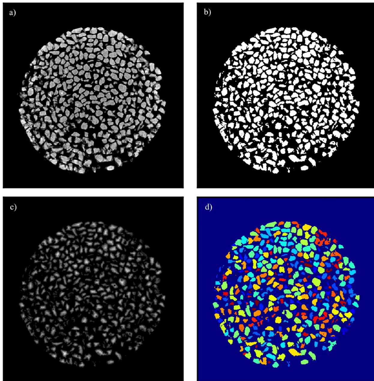
Fig. 4 Micro-CT image segmentation process. (a) Raw grayscale micro-CT image of silica sand. (b) A threshold operation is performed. (c) A distance transformation is applied. Pixel intensity corresponds with the distance to the nearest empty pixel. (d) A watershed algorithm is used to assign pixels to individual grains and labeled by color.
