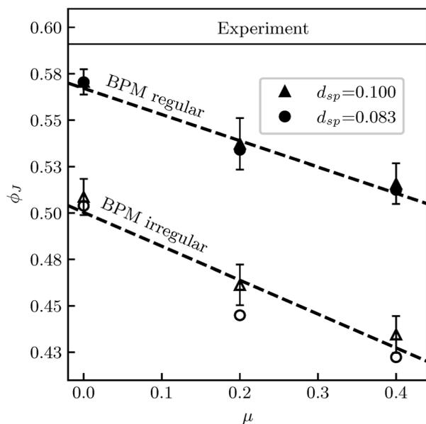
Fig. 14 Plot of jamming packing fraction versus  $\mu$  with regular-shaped (rough) BPM grains shown as solid symbols and irregular-shaped BPM grains shown as open symbols. Error bars show one standard deviation for  $d_{sp} = 0.100$  from the 5 replicates for regular-shaped and 10 replicates for irregular-shaped grains. The horizontal black line plotted at  $\phi_J = 0.591$  represents the laboratory experiments of Section 2.
