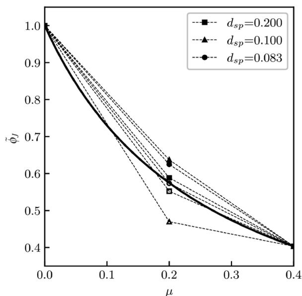
Fig. 16 Plot of  $\bar{\phi}_J$  (eqn (12)) versus  $\mu$ . The solid markers correspond to regular-shaped (rough) BPM grains while the hollow markers correspond to regular-shaped (smooth) BPM grains. The black line shows the relationship  $\bar{\phi}_J = 1/(1 + (\mu/\mu^*)^2)$ .
