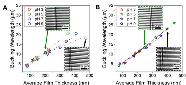
Fig. 4 Buckling wavelength of all LPAMA/LPMAA (A) and SPAMA/SPMAA (B) PEM films assembled from pH 3, 5, 7, and 9. Dashed linear trendlines are shown in all panels to guide the eye. Inset images show examples of wrinkles for pH 5 and pH 9 films, with a scale bar of 25 μm. The  $R^2$  values of the linear trendlines for panel A are 0.993 (pH 3), 0.998 (pH 5), 0.982 (pH 7), and 0.946 (pH 9). For panel B, the  $R^2$  values are 0.989 (pH 3), 0.997 (pH 5), 0.991 (pH 7), and 0.998 (pH 9).
