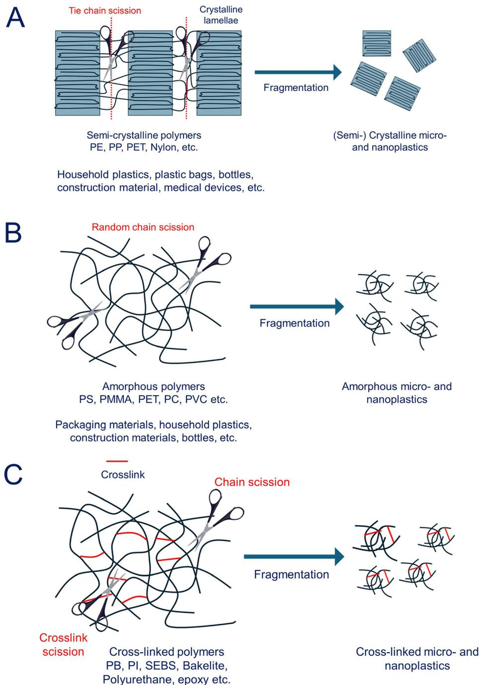
**Fig. 2** Mechanistic pathways of micro- and nanoplastic (MNPL) formation from bulk polymers. (A) (Semi-) Crystalline MNPL are predominantly expected to be formed as a result of tie-chain scission of semicrystalline polymers. (B) Amorphous plastics form micro- and nanoplastics by random scission of polymer chains into smaller fragments. (C) Cross-linked micro- and nanoplastics are formed by the fragmentation of cross-linked polymers such as rubbers and thermosets.
