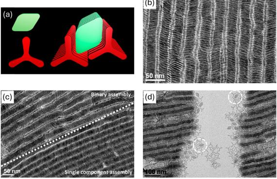
Fig. 25 (a) Schematic illustration of rhombic, tripodal nanoplates, and binary assembly. TEM images of (b) a binary co-assembly of tripodal and rhombic nanoplates formed via complementary-shape interaction, (c) a binary superstructure domain bordering a single-component superstructure domain of rhombic nanoplates, and (d) a fractured binary superstructure consisting of co-assembled tripodal and rhombic nanoplates. Adapted with permission from ref. 237. Copyright 2013 American Chemical Society.
