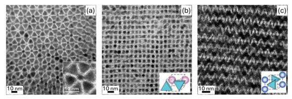
Fig. 18 TEM images of assemblies formed from LaF3 triangular nanoplates (9.0 nm side) and 5.0 nm Au nanoparticles on (a) silicon oxide surfaces or (b) on amorphous carbon substrates. (c) TEM image of an assembly formed from  $LaF_3$  triangular nanoplates (9.0 nm side) and 6.2 nm Au nanoparticles on amorphous carbon substrates. Insets: (a) magnified image; (b) and (c) proposed unit cells of the corresponding superstructures. Adapted with permission from ref. 31. Copyright 2006 Springer Nature
