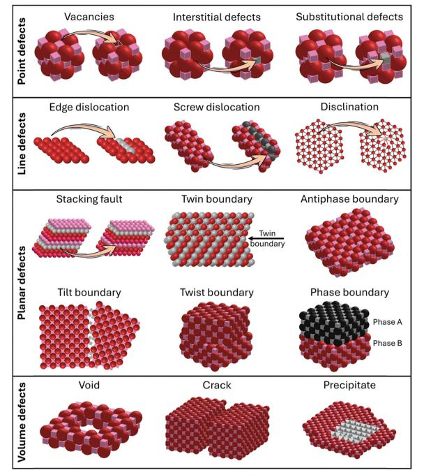
Fig. 3 Schematic representation of defects in a superstructure, including point defects (0D), line defects (1D), planar defects (2D), and volume defects (3D).
