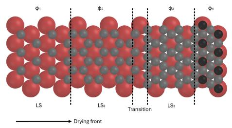
Fig. 33 Schematic illustration of the arrangement of small spheres onto a hexagonal layer of large spheres ( $\gamma \approx 0.5$ ), depending on the volume fraction. Adapted with permission from ref. 337. Copyright 2002 The American Association for the Advancement of Science.
