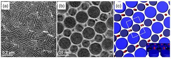
Fig. 28 (a) and (b) TEM images and (c) the structural model of an LMS-type superstructure co-assembled from small and large LaF<sub>3</sub> nanodisks and CdSe/ CdS nanorods. Adapted with permission from ref. 235. Copyright 2015 American Chemical Society.
