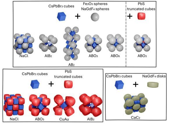
Fig. 20 Diversity of binary and ternary superstructures obtained from 5.3 and 8.6 nm cubic CsPbBr<sub>3</sub> nanoparticles combined with 11.2-25.1 nm spherical Fe<sub>3</sub>O<sub>4</sub> and NaGdF<sub>4</sub> nanoparticles, 10.7–11.7 nm truncated cuboid PbS nanoparticles, and NaGdF<sub>4</sub> disks (31.5 nm in diameter and 18.5 nm thick). Adapted with permission from ref. 240. Copyright 2022 American Chemical Society.
