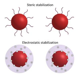
Fig. 2 Schematic representation of sterically and electrostatically stabilized nanometer- and submicrometer-sized particles
