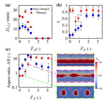
**Fig. 4** (a) The effective bubble diameter ( $D_{\rm eff}$ ) (b) correlation coefficient,  $\chi$ , and (c) aspect ratio (AR) for varying non-dimensional active matter force for a vibrated and non-vibrated gas-fluidized bed. The error bars are given as the standard deviation over the 8 s of pseudo steady-state simulation time.
