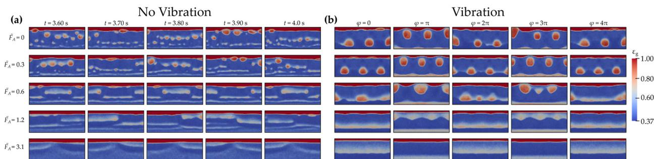
Fig. 3 Time-series of the void fraction in a gas-fluidized bed for varying non-dimensional active matter force which are (a) not vibrating or (b) vertically vibrating at  $f = 5$  Hz,  $\Gamma = 0.45$ , and  $A = 4.5$  mm.
