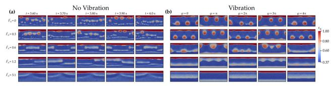
Fig. 3 Time-series of the void fraction in a gas-fluidized bed for varying non-dimensional active matter force which are (a) not vibrating or (b) vertically vibrating at f = 5 Hz,  $\Gamma = 0.45$ , and A = 4.5 mm
