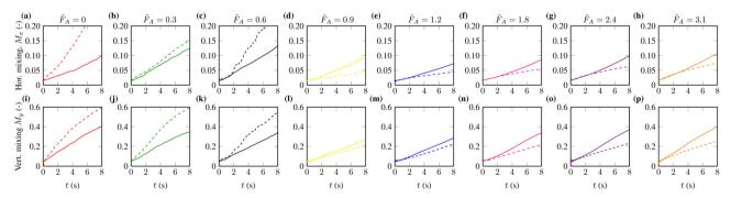
Fig. 10 Lacey mixing index over time in the horizontal direction,  $M_x$  (a)–(h) and the vertical direction,  $M_y$  (i)–(p) for the varying active matter force cases with no vibration (full lines) and vertical vibration (dashed lines). Note the difference in scale between the horizontal and vertical mixing indices
