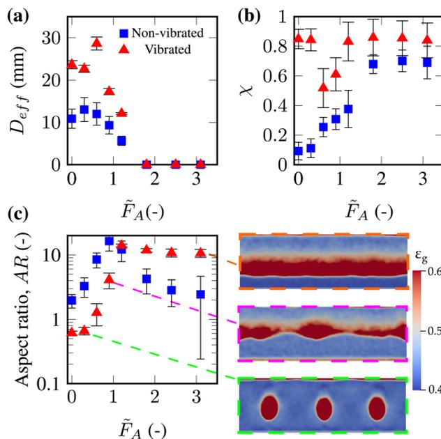
Fig. 4 (a) The effective bubble diameter ( $D_{\text{eff}}$ ) (b) correlation coefficient,  $\chi$ , and (c) aspect ratio (AR) for varying non-dimensional active matter force for a vibrated and non-vibrated gas-fluidized bed. The error bars are given as the standard deviation over the 8 s of pseudo steady-state simulation time.
