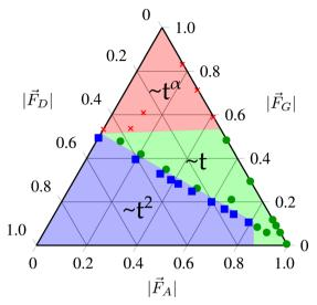
Fig. 7 A ternary diagram showing the dependence of the different mean squared displacement transport regimes (sub-diffusive MSD  $\sim t^{\alpha}$  where  $\alpha < 1$ , diffusion MSD  $\sim t$ , and advection MSD  $\sim t^2$ ) on the magnitude of the forces which act on particles (gravity  $|\vec{F}_G|$ , drag  $|\vec{F}_D|$ , and active matter force  $|F_A|$ ) relative to each other. Markers correspond to numerical simulations whilst shaded regions correspond to approximate transport regimes.
