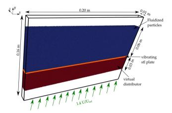
Schematic of the numerical simulation domain.
