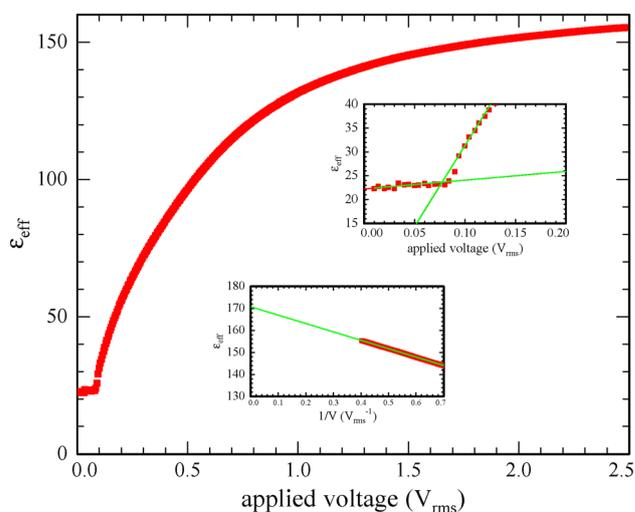
Fig. 3 Effective dielectric constant vs. voltage at 90 °C and 2.5 kHz. The upper inset shows the transition occurring at 0.076  $V_{\text{rms}}$ . The lower inset shows the extrapolation to infinite voltage enabling the determination of  $\epsilon_{\perp}$ .
