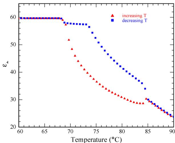
Fig. 11 Temperature dependence of  $\epsilon_{\perp}$  during both heating and cooling. Measured at 10 kHz and probe voltage of 0.05 V<sub>rms</sub>. Note the unusual kink at 73.3C, but only during cooling.
