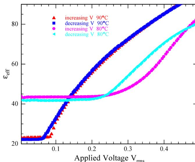
Fig. 9 Effective dielectric constants for both increasing and decreasing applied voltage in both the N and SmZ<sub>A</sub> phase; frequency 2.5 kHz.
