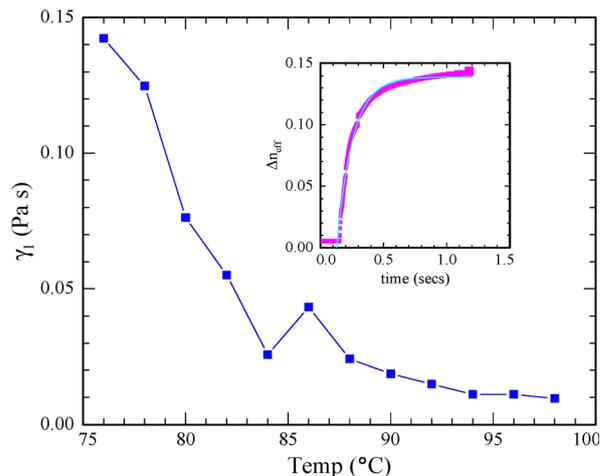
Fig. 6 Rotational viscosity vs. temperature. Inset: Example of change in effective birefringence vs. time after stepwise decrease in applied voltage. Green line shows fit to single exponential.
