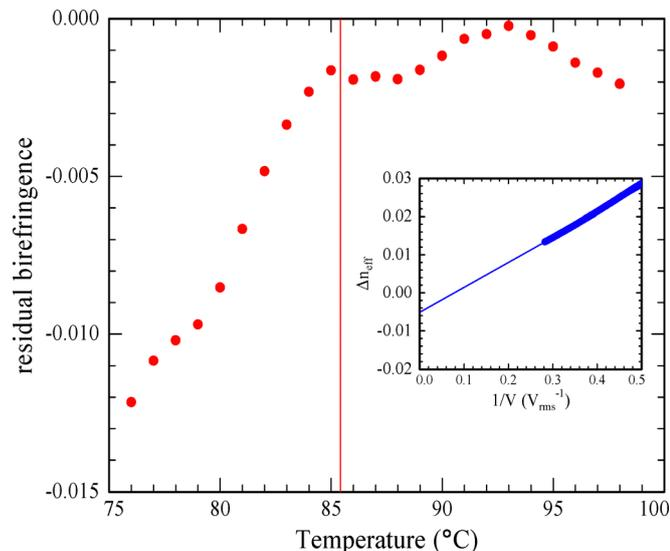
Fig. 7 Effective birefringence extrapolated to infinite potential difference vs. temperature. Vertical line is the N–SmZ<sub>A</sub> transition. Inset: Extrapolation example (corresponds to 80 °C).
