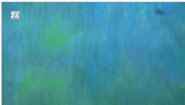
Fig. 12 POM image of DIO in Sm Z A phase right above threshold for magnetic FT. Periodic striations perpendicular to rubbing direction are observed (not seen in N phase).
