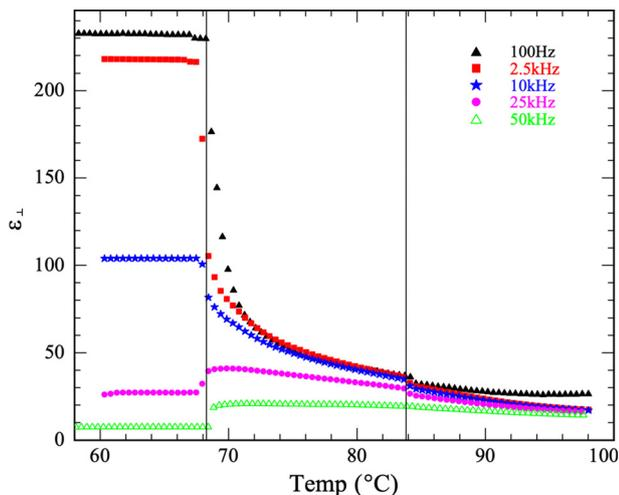
Fig. 1 Perpendicular component of dielectric constant vs. temperature at various frequencies. The vertical lines indicate the N–SmZ<sub>A</sub> and the SmZ<sub>A</sub>–N<sub>F</sub> phase transitions.
