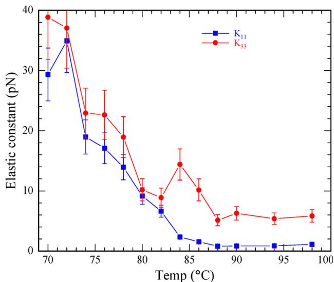
Fig. 5 Splay and bend elastic constants of DIO vs. temperature. Both increase dramatically at the N-SmZ<sub>A</sub> transition. The error bars reflect the uncertainty in determining both the threshold potential difference and the slope at onset (for K33).
