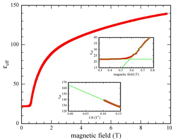
Fig. 4 Effective dielectric constant vs. magnetic field at 90 °C. The probe voltage is 0.004  $V_{\text{rms}}$  at 2.5 kHz. Upper inset shows close-up of FT; lower inset shows extrapolation to infinite magnetic field.
