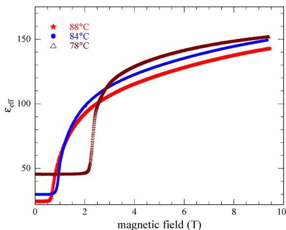
Fig. 8 Magnetic field induced FT at different temperatures above and below the N–SmZ<sub>A</sub> transition. No significant increase in rounding is seen below the transition temperature.
