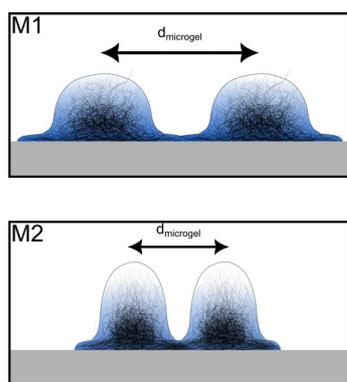
Fig. 11 Sketch of the effect of distance between microgels  $d_{\text{microgel}}$  on the structure and elastic response of the microgel monolayer. The microgels protrude further into the water for M2 because of the smaller microgel–microgel distance. The effect on the stiffness is represented by a different shading of the microgels in the vertical direction.
