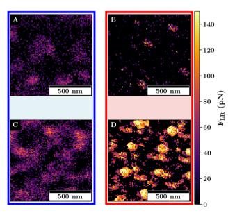
Fig. 8 Images of the long-range attractive interaction  $F_{LR}$  on monolayers M1 (A) and (B) and M2 (C) and (D) recorded at 27 °C (left) and at 40 °C (right). Measurements were recorded with a scan size of  $1 \times 1 \, \mu\text{m}^2$  and a resolution of  $80 \times 80$  pixels
