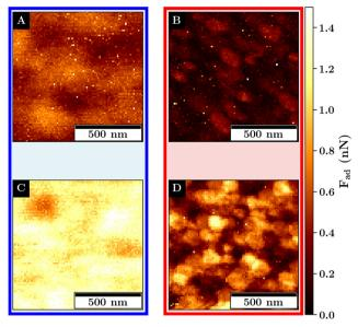
Fig. 7 Images of the adhesion force  $F_{ad}$  on monolayers M1 (A) and (B) and M2 (C) and (D) recorded at 27 °C (left) and at 40 °C (right). Measurements were recorded with a scan size of  $1 \times 1 \, \mu \text{m}^2$  and a resolution of  $80 \times 80$ pixels.
