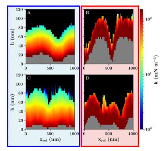
Fig. 10 Example stiffness profiles for monolayers M1 (A) and (B) and M2 (C) and (D). below (left) and above the VPTT (right). The black areas indicate a lack of stiffness data because the probe is not in contact with the sample. The grey areas indicate a lack of stiffness data for the set trigger threshold of 4 nN because the sample is not further deformed.
