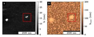
Fig. 1 Force volume measurement on a glass substrate with separated microgels recorded at 27 °C. (A) Height image and (B) corrected height image with a resolution of  $52 \times 52 \text{ px}^2$  and a scan size of  $5 \times 5 \text{ }\mu\text{m}^2$ . The red square represents the scan area used to measure the single probemicrogel interactions. The measurement was performed with a ramp speed of 10  $\mu m s^{-1}$ .
