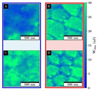
Fig. 12 Images of the dissipative energy on monolayers M1 (A) and (B) and M2 (C) and (D) recorded at 27 °C (left) and at 40 °C (right). Measurements were recorded with a scan size of  $1 \times 1 \,\mu\text{m}^2$  and a resolution of  $80 \times 80$ pixels.
