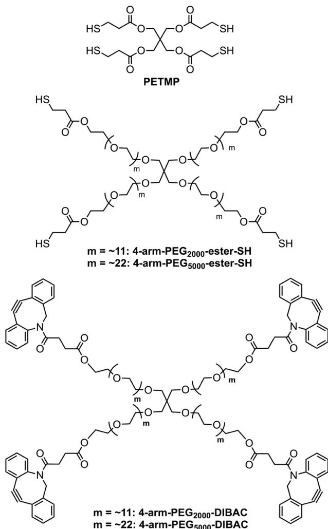
Fig. 2 Chemical structures of PETMP, 4-arm-PEG-ester-SH, and 4-arm-PEG-DIBAC.
