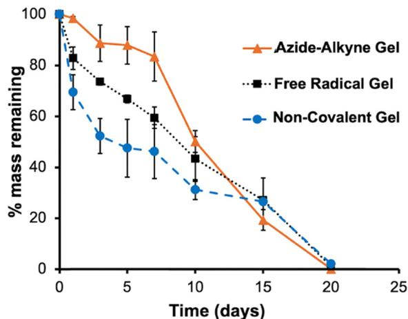
**Fig. 4** Degradation of the hydrogels loaded with 10% (w/w) ATRA as measured in PBS at 37 °C. The measurements were performed on triplicate samples of ATRA-loaded gels and the error bars correspond to the standard deviations.
