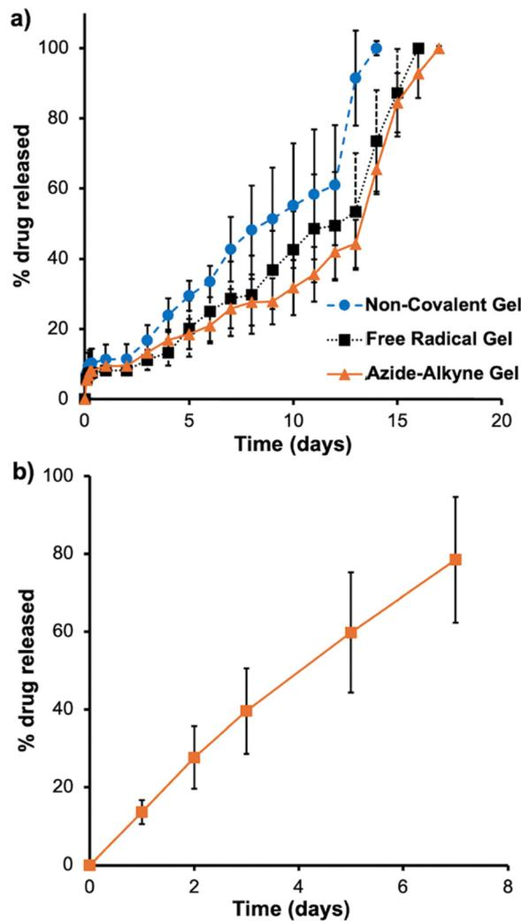
**Fig. 5** ATRA release from (a) the three different hydrogels in PBS with 2% (w/w) Tween 80 at 37 °C; (b) azide-alkyne gel in DMEM containing 10% fetal bovine serum at 37 °C. All measurements were performed on triplicate samples of ATRA-loaded gels, and the error bars correspond to the standard deviations.
