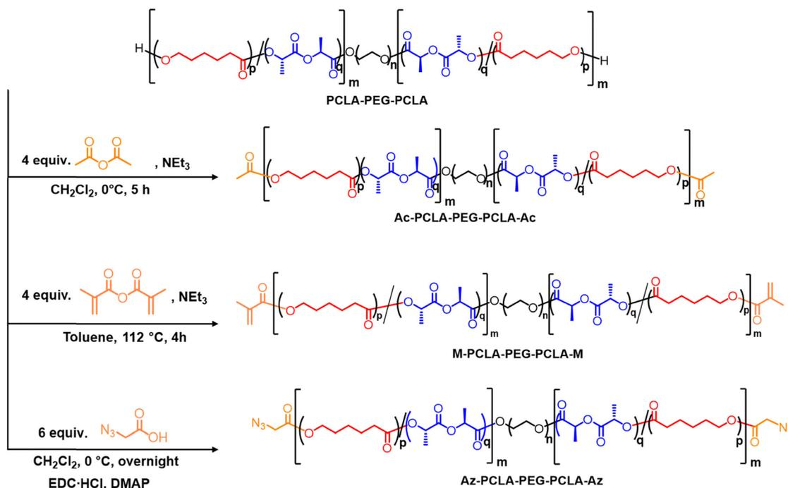
Scheme 1 Synthesis of the Ac-PCLA-PEG-PCLA-A, M-PCLA-PEG-PCLA-M and Az-PCLA-PEG-PCLA-Az.
