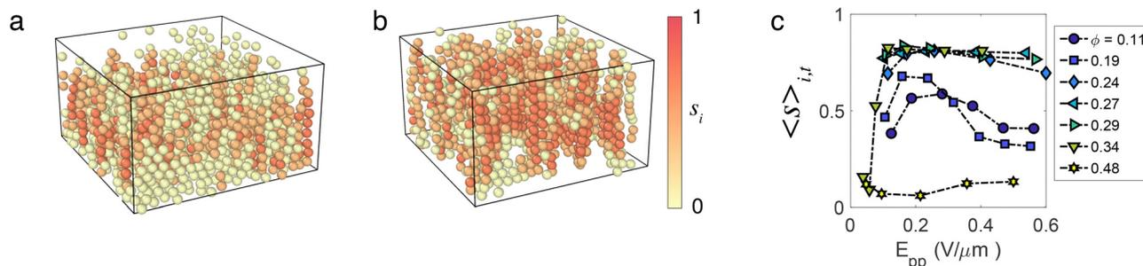
Fig. 2 Sheet structures. (a) and (b) 3D rendered snapshots of the sheet state ( $\phi = 0.1$ ) for  $E_{pp} = 0.13 \text{ V mm}^{-1}$  (a) and  $E_{pp} = 0.28 \text{ V mm}^{-1}$ . (b) Particles are coloured according to the value of their string order parameter  $\langle S_{i,t} \rangle_{i,t}$ . The average is taken over all particles  $i$  and time. (c) Mean string order parameter  $\langle S_{i,t} \rangle_{i,t}$  with respect to field strength  $E_{pp}$  and volume fraction  $\phi$ .
