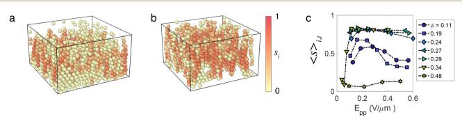
Fig. 2 Sheet structures. (a) and (b) 3D rendered snapshots of the sheet state ( $\phi = 0.1$ ) for  $E_{\rm pp} = 0.13$  V mm $^{-1}$  (a) and  $E_{\rm pp} = 0.28$  V mm $^{-1}$ . (b) Particles are coloured according to the value of their string order parameter  $(S_{i,t})_{i,t}$ . The average is taken over all particles i and time. (c) Mean string order parameter  $\langle S_{i,t} \rangle_{i,t}$  with respect to field strength  $E_{pp}$  and volume fraction  $\phi$ .
