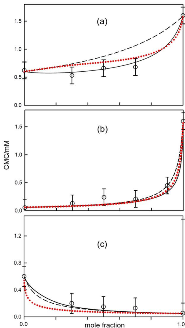
Fig. 4 Variation in cmc with solution composition for (a) LAS/AS, (b) LAS/LS and (c) LS/AS mixtures. The solid lines are model calculations using the PPA approach outlined earlier and for (black line) the parameters in Table 4, (red dotted line) parameters in Table 6, and (dashed line) ideal mixing.
