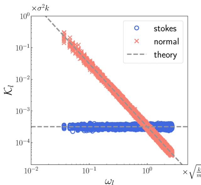
Fig. 1 The kinetic energy for each mode against the characteristic frequency. Symbols express the simulation results and lines represent the theoretical results eqn (18) and (21). Blue symbols are for the Stokes drag model and red symbols are for the normal dissipative force model. The law of equipartition of energy is violated for the later case.
