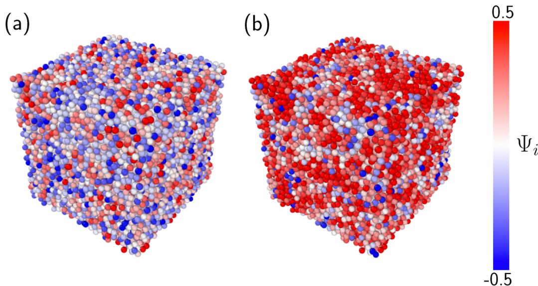
Fig. 2 Order parameter  $\Psi_i$  of the granular systems. Visualization of the spatial structure of the vibrations. Results for  $N = 16\,000$  are shown. (a) Stokes drag model and (b) normal dissipative force model. The color of the particles reflects the value of the order parameter, corresponding to the color bar on the right.
