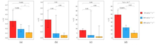
Fig. 11 Column plots (median and IQR) of the estimated MQLV parameters (a)  $\tau_1$ , (b)  $\tau_2$ , (c)  $\tau_3$  and (d)  $\tau_4$  for samples tested at 40 rad m<sup>-1</sup> s<sup>-1</sup> (red), 240 rad m<sup>-1</sup> s<sup>-1</sup> (blue) and 400 rad m<sup>-1</sup> s<sup>-1</sup> (orange). Also shown are the *p*-values obtained from Tukey multiple comparisons tests, with asterisks denoting a statistically significant difference (p < 0.05).
