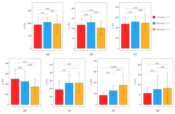
Fig. 10 Column plots (mean  $\pm$  SD) of the estimated MQLV parameters (a)  $\mu_0$ , (b)  $\mu_\infty$ , (c)  $c_2$ , (d)  $\mu_1$ , (e)  $\mu_2$ , (f)  $\mu_3$  and (g)  $\mu_4$  for samples tested at 40 rad m<sup>-1</sup> s<sup>-1</sup> (red), 240 rad m<sup>-1</sup> s<sup>-1</sup> (blue) and 400 rad m<sup>-1</sup> s<sup>-1</sup> (orange). Also shown are the *p*-values obtained from Tukey multiple comparisons tests, with asterisks denoting a statistically significant difference (p < 0.05).
