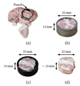
Fig. 1 Procedure for preparing cylindrical brain samples of radius 12.5 mm and height 10 mm for testing: (a) long cylindrical sample excised from the cerebral hemisphere using a steel punch; (b) top face cut flat using a cutting guide of height 13 mm; (c) opposite face cut flat using a cutting guide of height 10 mm and (d) flat cylindrical sample ready for testing.
