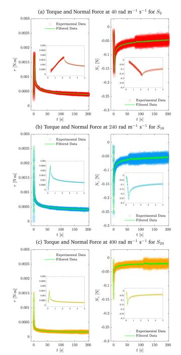
Fig. 5 Representative torque, normal force and filtered data for samples (a)  $S_{2}$ , (b)  $S_{16}$  and (c)  $S_{24}$  from torsion tests performed at twist rates of  $\{40,$ 240, 400) rad  $m^{-1}$  s<sup>-1</sup>. The insets show the ramp phase and the initial part of the hold phase in more detail.
