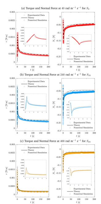
Fig. 7 Comparison of the resultant torque  $\tau$  and normal force  $N_{\tau}$  for samples (a)  $S_2$ , (b)  $S_{16}$  and (c)  $S_{24}$  at twist rates of {40, 240, 400} rad m<sup>-1</sup> s<sup>-1</sup>. Experimental data are denoted by circles, analytical predictions using the MQLV model by solid black lines and the results of the numerical simulations in FEniCS by triangles. The insets show the ramp phase and the initial part of the hold phase in more detail.
