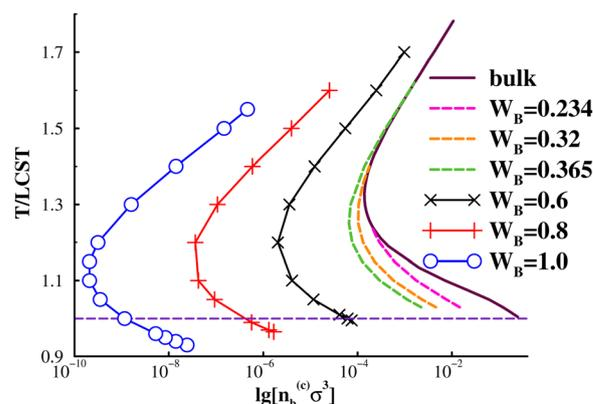
**Fig. 4** Prewetting lines for 300-mer polymer solution that displays an LCST.  $n_b^{(c)}$  denotes the bulk density at thin-thick coexistence. Upper prewetting temperatures,  $T_w(u)$  are obtained for three adsorption strengths:  $T_w(u, 0.234)/LCST \approx 1.24$ ,  $T_w(u, 0.32)/LCST \approx 1.41$ ,  $T_w(u, 0.234)/LCST \approx 1.62$ .
