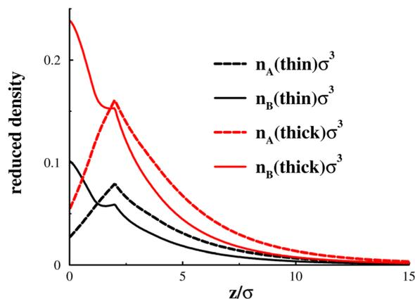
Fig. 5 Density profiles, for coexisting thin (black) and thick (red) phases, for a 300-mer solution, at the bulk LCST, with  $W_B^* = 0.6$ . Separate profiles for A (dashed) and B (solid) type are displayed.
