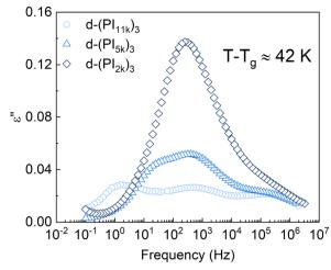
Fig. 4 Imaginary component of the dielectric permittivity for the different PI stars. For each sample, the selected temperature is about 42 K above its calorimetric  $T_{\rm o}$ .
