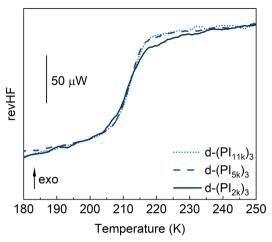
Fig. 9 Comparison of the reversing heat flow curves obtained by MDSC for the d-(PI) $_3$  stars during cooling at an average rate of 3 K min $^{-1}$ , a temperature oscillation amplitude of 0.5 K, and a period of 1 min.
