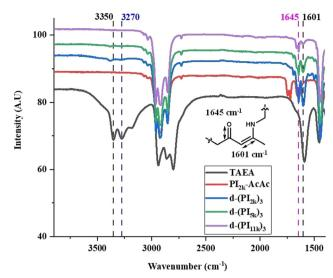
Fig. 2 FT-IR spectra of the linear precursor Pl2k-AcAc, TAEA, and the 3-arm PI stars [d-(PI)<sub>3</sub>] through vinylogous urethane chemistry.
