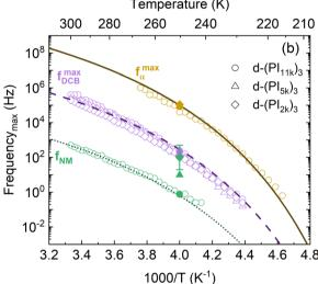
Fig. 5 Arrhenius plot of (a) the three peak maxima for the  $d-(Pl_{11k})_3$  star and (b) the peak maxima for the main components of each recorded spectrum (see text for details). Empty symbols correspond to the values obtained from visual inspection of the loss curves. Solid symbols correspond to the results obtained from the BDS data analysis using eqn (2). Lines correspond to the VFT description of these frequencies (see legend).
