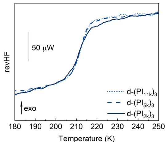
Fig. 9 Comparison of the reversing heat flow curves obtained by MDSC for the d-(PI)<sub>3</sub> stars during cooling at an average rate of 3 K min<sup>-1</sup>, a temperature oscillation amplitude of 0.5 K, and a period of 1 min.
