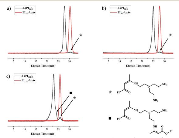
Fig. 1 SEC traces of 3-arm star PI [d-(PI)<sub>3</sub>] with molecular weight of PI-AcAc (a) 2 kg  $mol^{-1}$ , (b) 5 kg  $mol^{-1}$ , and (c) 11 kg  $mol^{-1}$  in THF at 35 °C.
