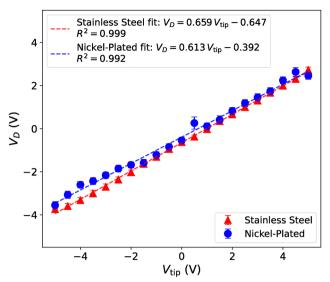
Fig. 4 Bias voltage applied to a 5 cm long, 2.69 mm ID syringe tip  $(V_{tip})$ versus the average voltage  $(V_D)$  of each drop, calculated using eqn (1). Error bars were produced from the standard deviation of n > 110 individual drops. Dashed lines depict linear fits to the data and are indicated in the legend. Data for the stainless steel tip and the nickel-plated tip were acquired at 49% and 34.5% RH, respectively.
