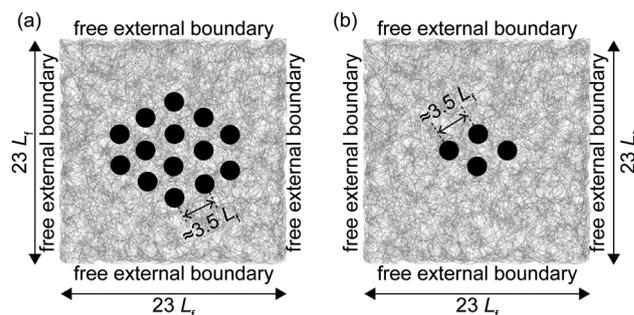
Fig. 1 Matrix with a cluster of inclusions. (a) A representative matrix containing a cluster of inclusions, each with a diameter of  $2L_f$ , spaced  $\approx 3.5L_f$  apart. (b) Simplified matrix model used in this study, showing a cluster with four inclusions, each spaced  $\approx 3.5L_f$  from their nearest neighbors. The inclusions first contracted simultaneously and then recovered, while the external edges of the matrix remained free.  $L_f$  denotes the average matrix fiber length.
