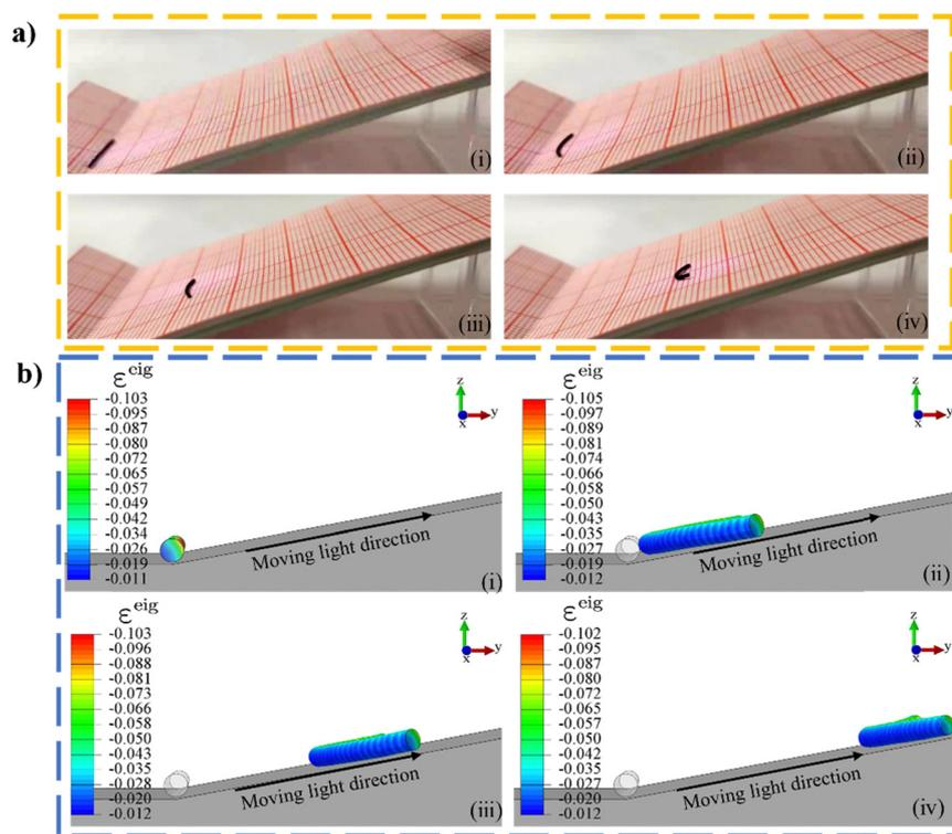
Fig. 5 Phototropic locomotion on an inclined surface. (a) Photographs from the experiments in ref. 15; (b) FE simulation. The experimental and FE parameters are: length 13 mm, diameter 0.58 mm,  $E = 10$  MPa,  $\rho = 10^6$  kg m $^{-3}$ . See also the supplementary animations (ESI†).
