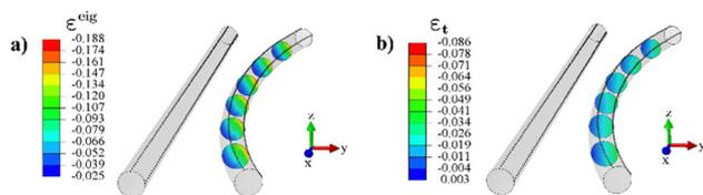
Fig. 3 (a) Eigenstrain and (b) geometric strain distribution along longitudinal direction  $\mathbf{t}$  when the cylindrical robot responds to photo illumination of incidence  $\theta = \pi/4$  by bending to the right in the  $x$ - $y$  plane. The FE parameters are as follows: length 13 mm, diameter 0.58 mm, Young's modulus  $E = 10$  MPa, density  $\rho = 10^6$  kg m<sup>-3</sup>, axial thermal expansion coefficient  $\alpha_t^0 = -0.19$ .
