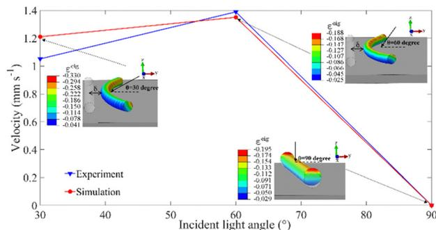
Fig. 11 Comparison between experiment<sup>47</sup> and simulation on the relation between light-induced rolling velocity and incident light angle. The experimental and FE parameters are: length 13 mm, diameter 0.58 mm,  $E = 10$  MPa,  $\rho = 1.1 \times 10^6$  kg m<sup>-3</sup>; the incident light angle is 30 degree, 60 degree, 90 degree respectively.
