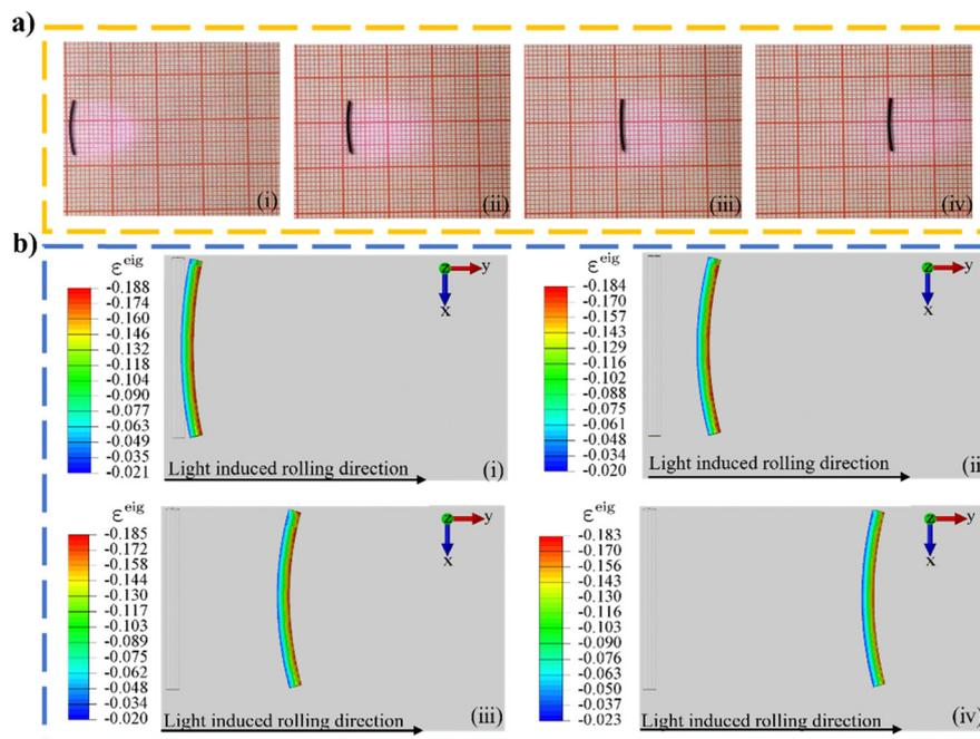
Fig. 4 Phototropic locomotion on a horizontal plane. (a) Photographs captured during the locomotion from the experiments in ref. 15; (b) FE simulation. The experimental and FE parameters are: length 13 mm, diameter 0.58 mm,  $E = 10$  MPa,  $\rho = 10^6$  kg m $^{-3}$ . See also the supplementary animations (ESI†).
