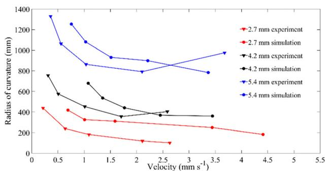
Fig. 9 Comparison between experiment<sup>47</sup> and simulation: on the relation between rolling velocity and radius of curvature for thermally induced rolling LCE rods. The experimental and FE parameters are as follows: length 70 mm,  $E = 5$  MPa,  $\rho = 10^3$  kg m<sup>-3</sup>, the diameter is 2.7 mm, 4.2 mm, 5.4 mm respectively.
