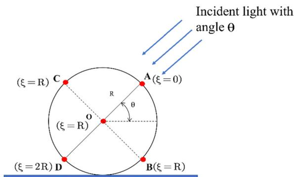
Fig. 2 Illustration of light incident on a circular cross section of the cylindrical robot of radius  $R$ .  $\theta$  is the angle between the incident light and the horizontal. The light propagation depth  $\xi$  through the material is measured along the direction of the incident light.
