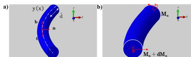
Fig. 1 Illustration of a stimuli-bent soft cylindrical robot. (a) Entire soft cylindrical robot under global  $(x, y, z)$  and  $(\mathbf{t}, \mathbf{n}, \mathbf{b})$  local coordinate systems. (b) Bending moments  $M_n$  and  $M_n + dM_n$  acting on a bent differential element of the cylinder.
