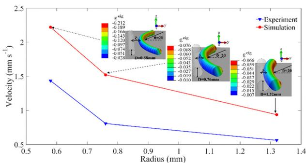
Fig. 12 Comparison between experiment<sup>47</sup> and simulation on the relation between light-induced rolling velocity and radius of LCE rods. The experimental and FE parameters are: length 13 mm,  $E = 10$  MPa,  $\rho = 1.1 \times 10^6$  kg m<sup>-3</sup>; the diameter is 0.58 mm, 0.76 mm and 1.32 mm respectively.
