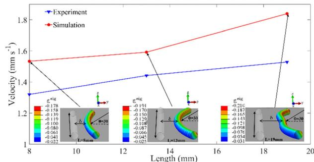
Fig. 13 Comparison between experiment<sup>47</sup> and simulation on the relation between light-induced rolling velocity and length. The experimental and FE parameters are: diameter 0.58 mm,  $E = 10$  MPa,  $\rho = 1.1 \times 10^6$  kg m<sup>-3</sup>, the length is 8 mm, 13 mm and 19 mm respectively.
