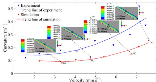
Fig. 10 Comparison between experiments<sup>48,49</sup> and simulations on the relation between heat-induced rolling velocity and curvature of a nylon fibre. The experimental and FE parameters: length 130 mm, diameter 0.6 mm,  $E = 100$  MPa,  $\rho = 1.1 \times 10^3$  kg m<sup>-3</sup>.
