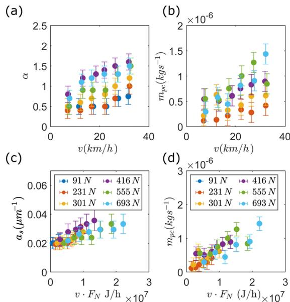
Fig. 3 Variation of  $\alpha$  (a) and the total mass  $m_{\text{pc}}$  (c) of the particles, as measured by the particle counter, are shown as a function of velocity  $v$  for different values of the normal force  $F_N$ . The specific surface area  $a_s$  (b) and  $m_{\text{pc}}$  (d) for the small MNPs are found to scale with the product of velocity  $v$  and normal force  $F_N$ .
