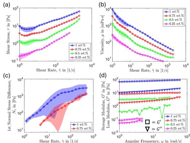
Fig. 2 Rheological measurements for different concentrations of MFC suspensions showing (a) shear stress versus shear rate, (b) viscosity versus shear rate, (c) first normal stress difference versus shear rate, and (d) storage and loss moduli versus angular frequency.
