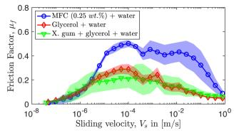
Fig. 6 Tribological friction factor as a function of sliding velocity for 0.25 wt% MFC suspension, 0.3 wt% xanthan gum in 50:50 wt% glycerolwater solution and 60:40 vol% glycerol-water mixture.
