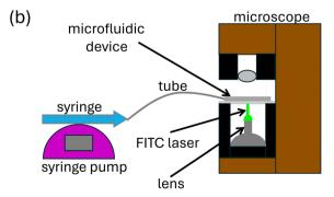
Fig. 3 (a) Diagram showing the basic design of the microchannel used in this study. (b) The general setup of the experiments.
