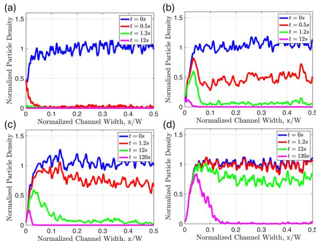
Fig. 8 Results for the particle density profile as a function of channel width at different times for (a)  $\phi = 1$  wt%, (b)  $\phi = 0.75$  wt%, (c)  $\phi = 0.5$  wt%, and (d)  $\phi = 0.25$  wt%. All experiments shown were performed at a shear rate  $\dot{\gamma} \approx 1300 \text{ s}^{-1}$ .
