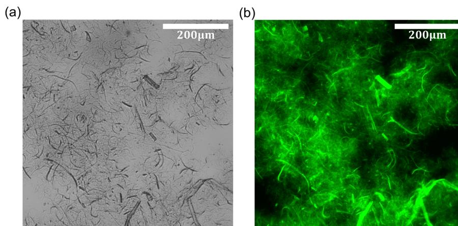
Fig. 1 Images of micro fibrillated cellulose (MFC)-water suspension at 1 wt% concentration using a 20 $\times$  objective magnification in (a) bright-field microscopy and (b) fluorescence microscopy. The green represents fiber-rich regions whereas the black represents the surrounding solvent (water).
