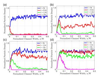
Fig. 8 Results for the particle density profile as a function of channel width at different times for (a)  $\phi=1$  wt%, (b)  $\phi=0.75$  wt%, (c)  $\phi=0.5$  wt%, and (d)  $\phi=0.25$  wt%. All experiments shown were performed at a shear rate  $\dot{\gamma}\approx1300$  s<sup>-1</sup>.
