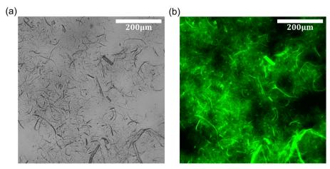
Fig. 1 Images of micro fibrillated cellulose (MFC)-water suspension at 1 wt% concentration using a 20× objective magnification in (a) bright-field microscopy and (b) fluorescence microscopy. The green represents fiber-rich regions whereas the black represents the surrounding solvent (water).
