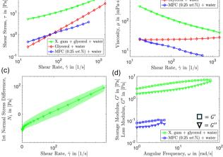
Fig. 5 Rheological measurements for control fluids, 0.3 wt% xanthan gum in glycerol and water (50:50 wt%) and glycerol and water solutions (60:40 vol%) compared to 0.25 wt% MFC in water suspension showing (a) shear stress versus shear rate, (b) viscosity versus shear rate, (c) first normal stress difference versus shear rate, and (d) storage and loss moduli versus angular frequency.
