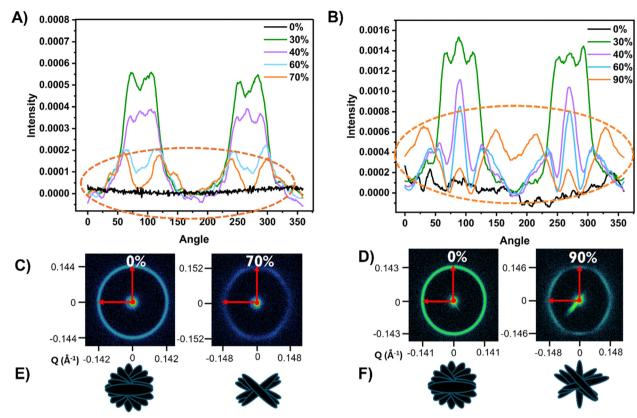
Fig. 7 (A) SAXS intensity vs. angle of 50 μm thick (A) visible and (B) MWIR reflective CLCEs under strain. SAXS scattering patterns of a (C) visible CLCE at 0% and 70% strains and (D) of a MWIR CLCE at 0% and 90% strains. Depictions of the LC director reorientation and distortion is represented for (E) visible and (F) MWIR reflective CLCEs before and after strain.
