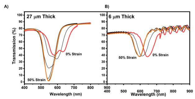
Fig. 2 CLCEs were prepared with reflection notches at approximately 600 nm that were (A) 27 μm thick and (B) 6 μm thick and subject to 0-50% strain at 10% strain increments.
