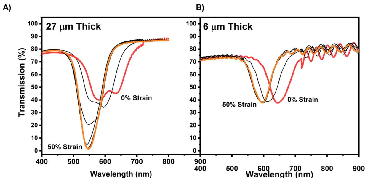
**Fig. 2** CLCEs were prepared with reflection notches at approximately 600 nm that were (A)  $27\ \mu\text{m}$  thick and (B)  $6\ \mu\text{m}$  thick and subject to 0–50% strain at 10% strain increments.
