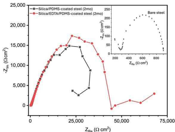
Fig. 8 Nyquist plot comparing aged-coated samples and bare metal, where the x-axis represents the real part of the impedance, and the y-axis shows the imaginary part of the impedance, capturing resistive and capacitive/inductive behaviors, respectively.
