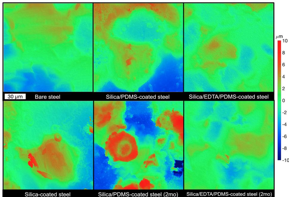
Fig. 5 Heightmaps of the six different surfaces investigated in this study. "2mo" denotes surfaces imaged two months after coating deposition.
