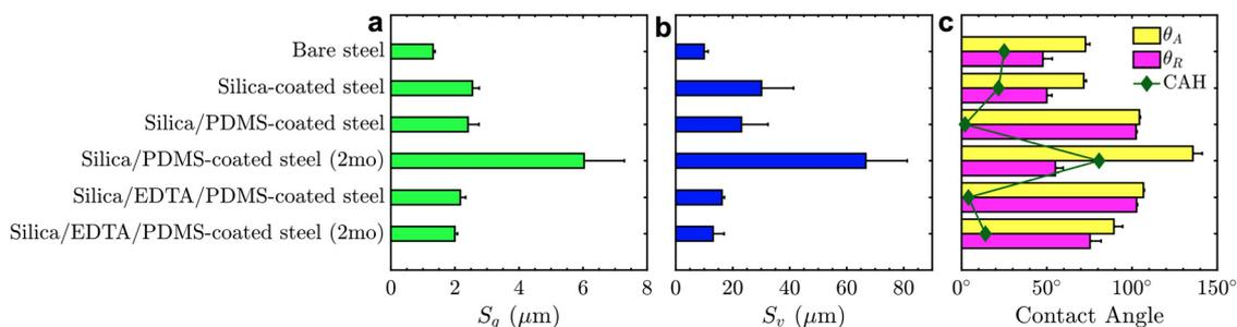
Fig. 6 3D laser scanning microscope measurements of (a)  $S_q$  (root-mean-squared roughness) and (b)  $S_v$  (maximum valley depth) of the bare and coated steel surfaces. (c) Advancing water contact angle, receding water contact angle, and contact angle hysteresis of the same surfaces.
