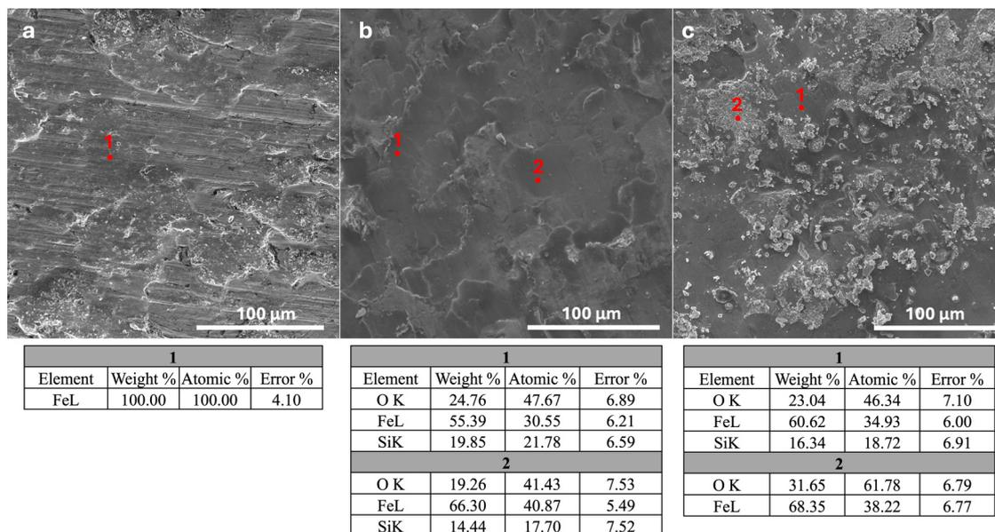
Fig. 3 SEM images and EDS analyses of (a) bare carbon steel, (b) silica/EDTA/PDMS-coated carbon steel, and (c) corroded silica/EDTA/PDMS-coated carbon steel imaged 1.5 years after coating deposition. Numbered spots show areas where EDS data were collected, with results displayed in the tables below each corresponding image.
