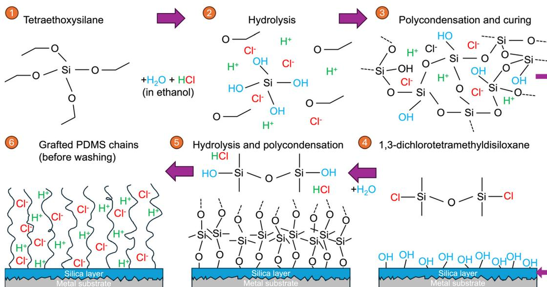
**Fig. 1** Typical route of silica layer deposition (steps 1–3) and omniphobic PDMS grafting to the silica layer using chlorosilanes (steps 4–6). Chlorides are present throughout both processes. Note the schematics are not to scale, and typically the silica layer is  $\sim 300$  nm thick,<sup>9</sup> whereas the omniphobic PDMS is around 4 nm thick.<sup>8</sup>
