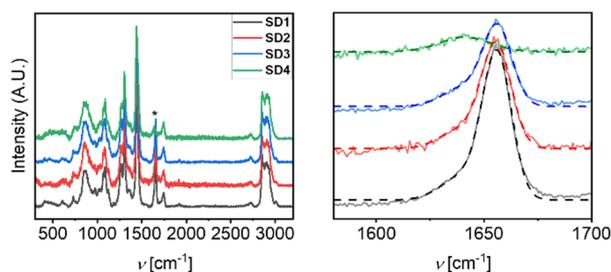
Fig. 3 Raman analysis of the cured SD 1 to SD 4 gels. Left: Traces overlay. Right zoom in in the region between  $1580$  and  $1700\text{ cm}^{-1}$  of the RAMAN curves (full lines) related to both  $\text{C=C}$  and oxazolidone stretching frequencies and fitting according to Gaussian extrapolation (peaks at  $1640$  and  $1656\text{ cm}^{-1}$ , dotted lines).
