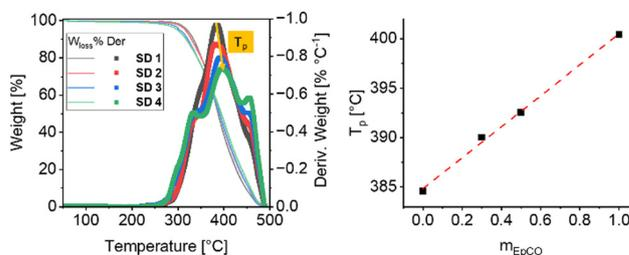
Fig. 5 TGA analysis of the SD 1 to SD 4 samples. Left: Weight loss (line) and derivative weight loss curves (dots) and depiction of the derivative peak temperature ( $T_p$ ) of the more intense degradation step. Right: Evolution of  $T_p$  over mass fraction of EpCO over CO; the dotted line is a guide.
