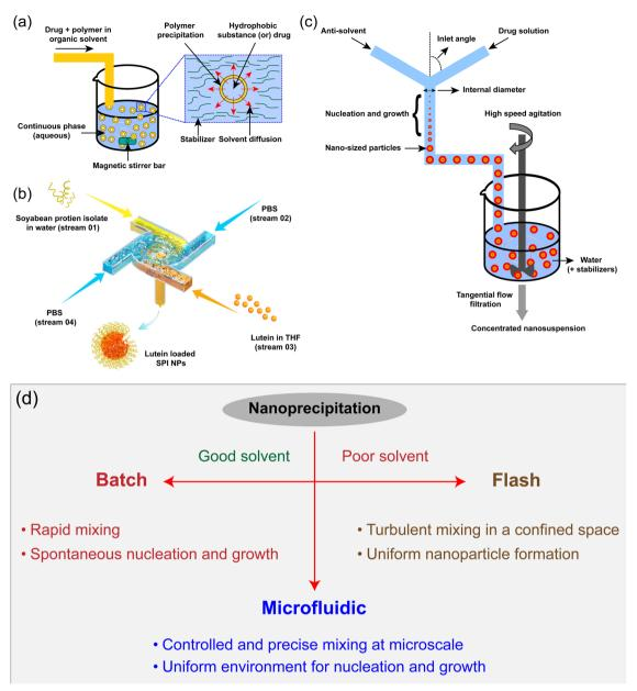
Fig. 2 Major types of mixing processes for nanoprecipitation. (a) Batch nanoprecipitation (BNP),<sup>48</sup> (b) flash nanoprecipitation (FNP),<sup>51</sup> and (c) microfluidic nanoprecipitation (MNP),<sup>52</sup> (d) principles of batch, flash, and microfluidic nanoprecipitation techniques.
