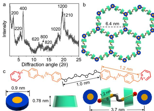
**Fig. 1** (a) XRD pattern of the ISF xerogel, (b) corresponding simulated structure showing side spacing in *ab* plane, and (c) analysis of the framework structure in reference to the sizes of the  $\text{AlMo}_6^{3-}$  and  $\text{CPR}^{2+}$  components.
