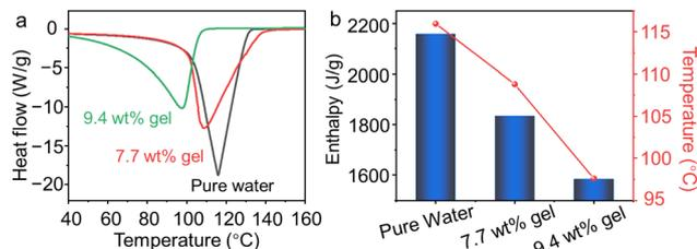
Fig. 3 (a) Plots of heat flow versus temperature for pure water and ISF hydrogels (7.7 wt% and 9.4 wt%), and (b) evaporation enthalpies of pure water and ISF hydrogels (7.7 wt% and 9.4 wt%).
