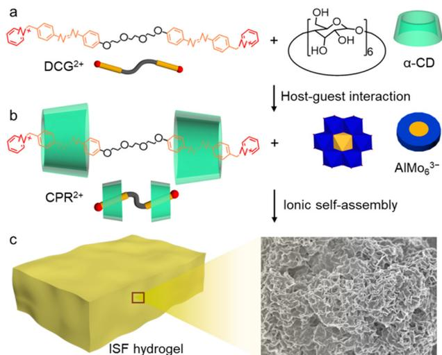
**Scheme 1** Schematic chemical structures and representations of (a) the building blocks of the developed hydrogel, namely di-cationic guest DCG·2Br and host molecule  $\alpha$ -CD, (b) pseudo-rotaxane component (CPR·2Br) and POM cluster  $\text{AlMo}_6^{3-}$ , and (c) formation of ISF hydrogel via ionic self-assembly, with its SEM image also shown.
