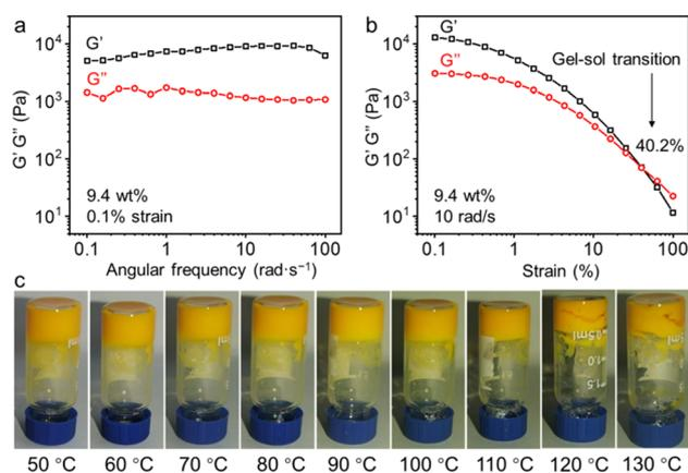
Fig. 2 (a) Plots showing the rheology of the prepared ISF hydrogel as a function of angular frequency, (b) strain analysis of the hydrogel, and (c) photographs showing the hydrogel stability from 50 °C to 130 °C.
