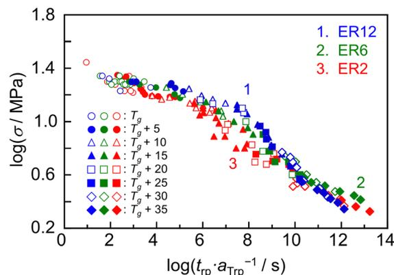
Fig. 5 Master curves of the  $t_{rp}$ - $\sigma$  plots for ER12, ER6 and ER2 after horizontal shifting. Blue, green, and red-colored symbols denote the data for ER12, ER6, and ER2, respectively. The reference temperature was set to  $T_g$ .
