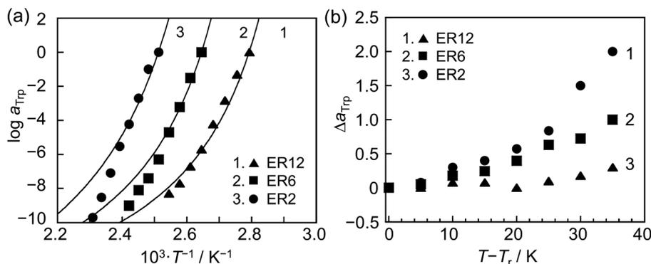
Fig. 6 (a) Temperature dependence of  $a_{TTP}$  for ER2, ER6, and ER12. Closed symbols denote experimental data, and solid curves indicate the best-fit WLF equation applied to the  $a_T$ - $T$  relationship from the creep test. (b) Correlation between  $\Delta a_{TTP}$  and  $\Delta T$  ( $T - T_f$ ).
