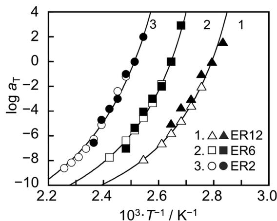
**Fig. 3** Temperature dependence of  $a_T$  for ER12, ER6 and ER2. Closed symbols represent experimental data obtained from the creep test, while open symbols correspond to data from DMA measurements. Solid curves indicate the best fit of the WLF equation to the DMA data. (The DMA data are reproduced from ref. 65 with permission. Copyright 2021 American Chemical Society).
