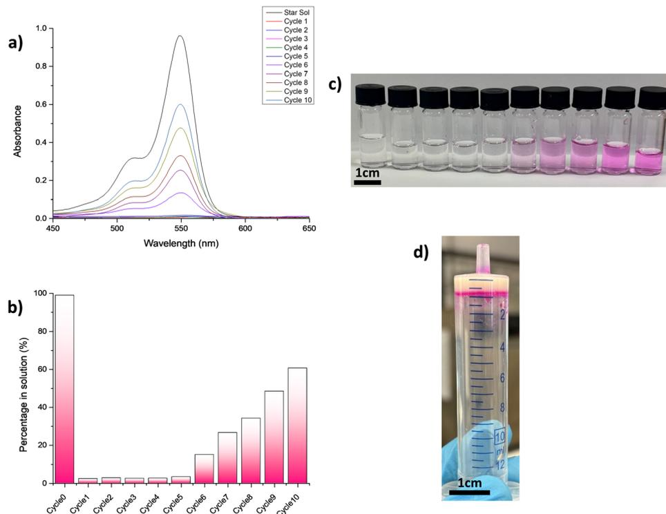
Fig. 5 (a) Absorbance spectra of filtered solution of RB ( $1.1 \times 10^{-5}$  M starting solution), (b) histogram of dye amount in the filtered solution, (c) colour change of filtered solutions (scale bar of 1 cm) and (d) inversion tube test of **L1** gel in DMSO : H<sub>2</sub>O (1 : 1 v/v) at 1% w/v after RB removal (scale bar of 1 cm).
