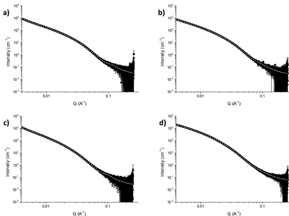
Fig. 3 (a) SAXS data for gel **L1** in DMSO:H<sub>2</sub>O (3:7 v/v) at 0.5% w/v, (b) SAXS data for **L1** (DMSO:H<sub>2</sub>O (2:3 v/v) at 1% w/v), (c) SAXS data for **L1** DMSO:H<sub>2</sub>O (1:1 v/v) at 1% w/v and (d) SAXS data for **L1** DMSO:H<sub>2</sub>O (1:1 v/v) at 2% w/v.
