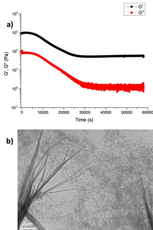
**Fig. 2** (a) Time sweep of gel **L2**, DMSO:H<sub>2</sub>O (1:1 v/v) at 0.5% w/v, (b) TEM images (scale bar of 2 μm) that show the presence of different size fibers.
