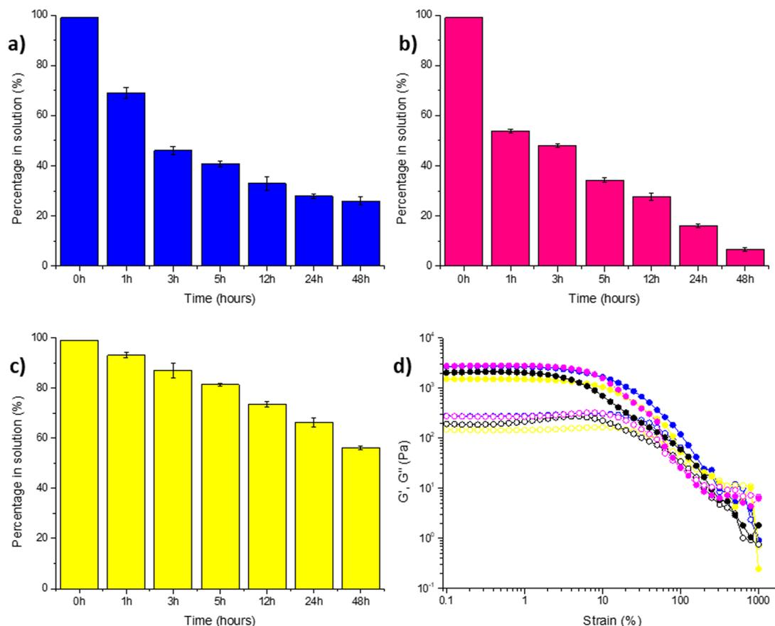
Fig. 4 Histograms of dye adsorption results for **L1** in DMSO : H<sub>2</sub>O (3 : 7 v/v), 0.5% w/v in the presence of (a) NB, (b) RB, (c) NY and (d) strain sweep of **L1** in DMSO : H<sub>2</sub>O (3 : 7 v/v) at 0.5% w/v after dye adsorption (full points indicate  $G'$  and empty points indicate  $G''$ , black points represent free gels, blue points represent gels in the presence of NB, yellow points represent gels in the presence of NY and pink points represent gels in the presence of RB).
