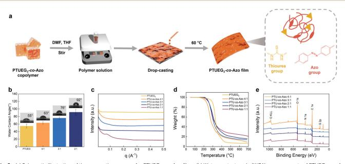
Fig. 2 (a) Schematic illustration of the preparation process for  $PTUEG_{\pi}$ -co-Azo films. (b) Water contact angle (WCA) measurements of  $PTUEG_{\pi}$ -co-Azo films. (c) Small-angle X-ray scattering (SAXS) profiles of PTUEG3 and PTUEG3-co-Azo films with different TUEG-DA: Azo-DA ratios (1:1, 2:1, 3:1, and 4:1). (d) Thermogravimetric analysis (TGA) curves of PTUEG3 and PTUEG3-co-Azo films. (e) XPS survey spectra of PTUEG3-co-Azo films.
