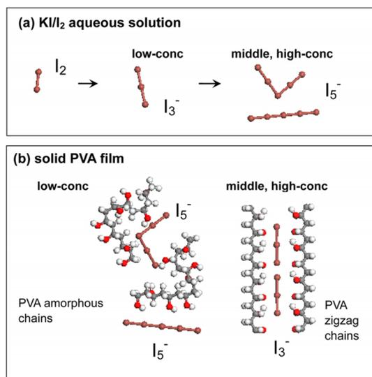
Fig. 10 Schematic of iodine species in (a) iodine solution, (b) solid PVA film, showing its distribution in the amorphous and crystalline regions of a PVA sample dipped in KI/I<sub>2</sub> solutions of different concentrations. Reprinted with permission from ref. 110; copyright 2015, the American Chemical Society.
