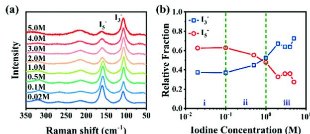
Fig. 11 (a) Raman spectra of PVA films dipped in KI/I<sub>2</sub> with different iodine concentrations. (b) Relative fraction of  $I_3^-$  and  $I_5^-$  obtained from peak deconvolution. Reprinted with permission from ref. 115; copyright 2021, the Royal Society of Chemistry.
