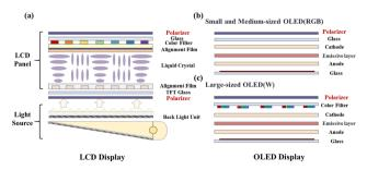
Fig. 1 Schematic of the panel structure: (a) LCD panel, (b) small- and medium-sized OLED and (c) large-sized OLED
