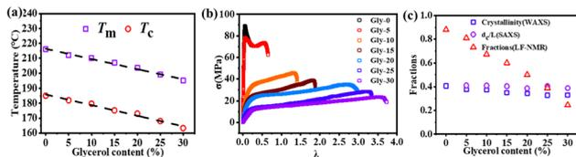
**Fig. 8** (a) Summary of  $T_m$  and  $T_c$  dependence of the glycerol content and the linear fitting of  $1/T_m$  and  $1/T_c$ . (b) Stress–strain curves of PVA films with different addition ratios of glycerol. (c) Comparison of the crystallinity obtained from WAXS ( $\chi_c$ ), SAXS ( $d_c/L$ ), and NMR ( $f_c$ ) experiments. Reprinted with permission from ref. 91 copyright 2023, John Wiley and Sons.
