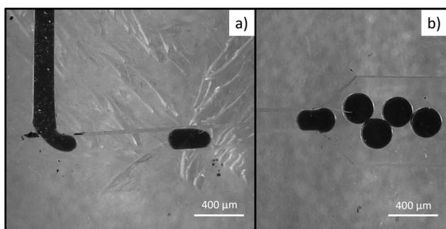
Fig. 2 Two particle morphologies were determined within the microfluidic system. (a) In the  $D_s$  channel area the particle takes on a plug-like shape governed by the interfacial tensions of disperse and continuous phase. (b) After the widening of the downstream channel the microparticle shape is disc-like, confined by the upper and lower channel walls.
