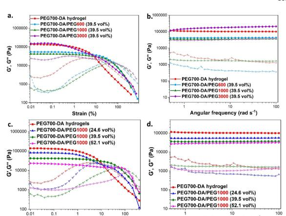
Fig. 3 (a) and (b) Amplitude and frequency sweeps of PEG700-DA/PEGx (39.5 vol%) examining the effect of PEG's molecular weight. (d) and (e) Amplitude and frequency sweeps of PEG700-DA/PEG1000 hydrogels examining the effect of PEG's vol%. Experiments were conducted at 37 °C using an oscillatory mode where storage modulus (G', filled symbols) and loss modulus (G', empty symbols).
