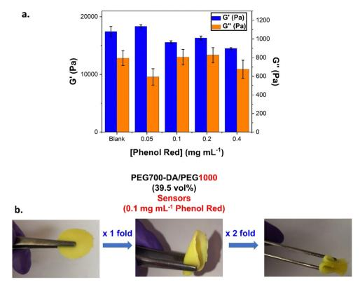
Fig. 6 (a) Viscoelastic data for formulations containing various phenol red concentrations (b) PEG700-DA/PEG1000 (39.5 vol%) sensor gels containing  $0.1 \text{ mg mL}^{-1}$  phenol red with high tolerance to deformation.
