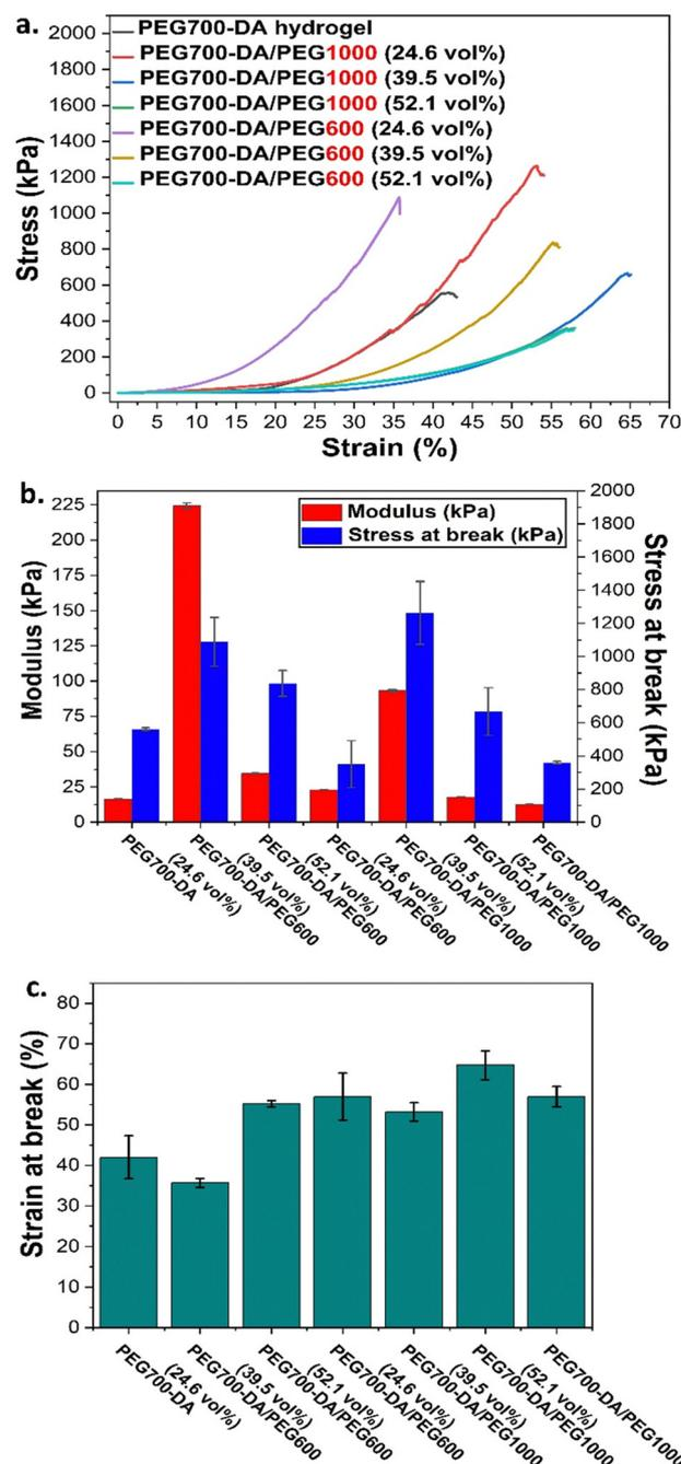
Fig. 2 (a) Representative compression curves for pristine PEG700-DA/PEGx hydrogels (b) modulus and stress at break data and (c) strain at break results. Data given as mean  $\pm$  SD of the average of at least  $n = 8$  samples.
