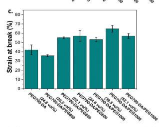
Fig. 2 (a) Representative compression curves for pristine PEG700-A/ PEGx hydrogels (b) modulus and stress at break data and (c) strain at break results. Data given as mean  $\pm$  SD of the average of at least n=8 samples.
