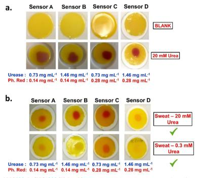
Fig. 7 (a) Control experiments of PEG700-DA/PEG1000 (39.5 vol%) sensors containing various concentrations of urease and phenol red before (blank) and after exposure to 20 µL of 20 mM urea solution. Images taken after 10 min of exposure. (b) Images from PEG700-DA/PEG1000 (39.5 vol%) sensors containing various concentrations of urease and phenol red exposed to 20 µL of two different model sweat formulations containing 0.3 and 20 mM of
