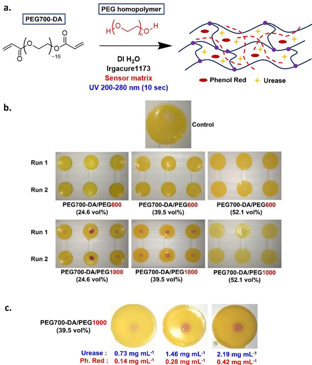
**Fig. 5** (a) General schematic of hydrogel sensor synthesis, (b) sensor tests with 20  $\mu\text{L}$  of urea (0.002, 0.015 and 0.02 M from left to right) in duplicates with formulations containing 0.73  $\text{mg mL}^{-1}$  of urease and 0.14  $\text{mg mL}^{-1}$  of phenol red in duplicates, (c) PEG700-DA/PEG1000 (39.5 vol%) sensor tests with varying amounts of urease and phenol red using 20  $\mu\text{L}$  of 0.02 M urea.
