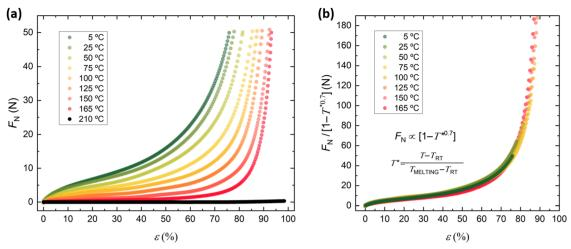
Fig. 4 Temperature dependency of 650-μm single  $Sn_{63}Pb_{37}$  balls. (a) Force-strain relation at different temperatures in the range 5–210 °C. A constant strain rate of  $4.0 \times 10^{-4}$  s<sup>-1</sup> was used. (b) The normalized force-strain relation reveals that a temperature-dependent scaling factor  $1 - T^{*m}$  can be used to describe the behavior, with the parameter m determined to be 0.7. The results indicate a strong dependence of force on temperature.
