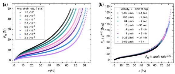
Fig. 3 Strain rate dependency of 650- $\mu$ m single Sn<sub>63</sub>Pb<sub>37</sub> solder balls. (a) Force-strain relation at different strain rates varying from 3.1 × 10<sup>-5</sup> to 1.5 s<sup>-1</sup>. (b) The normalized force-strain relation reveals that a simple power-law relation can be used to scale the force. The power-law exponent of 0.12 indicates a very weak dependence of force on strain rate.
