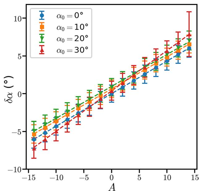
Fig. 2 Variations of the angle  $\delta\alpha$  as a function of the applied tangential force  $A$  averaged over 200 trajectory frames for different values of the nominal angle  $\alpha_0$ . The linear regressions are plotted as dashed lines. Error bars correspond to the standard deviations of  $\delta\alpha$ .
