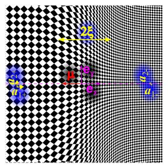
Fig. 2 Magnetic pattern (top view). The magnetization of the pattern follows eqn (1) with the modulus given by eqn (2). The larger lattice constant is  $a_{+} = 21 \,\mu\text{m}$ , the magnification factor is  $m = 3 \,(a_{-} = 7 \,\mu\text{m})$ , and the transition length is  $\xi = 75 \,\mu\text{m}$ .
