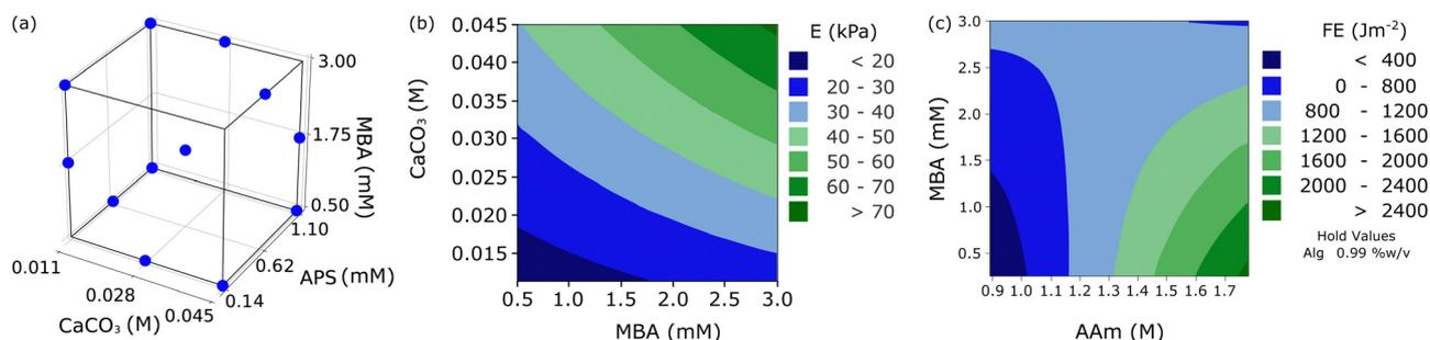
**Fig. 3** (a) A schematic representation of the fractional factorial design approach used for secondary screening; (b) contour plot showing the effect of MBA and  $\text{CaCO}_3$  on  $E$ ; (c) contour plots of the predicted values of FE, derived from secondary screening for different concentrations of MBA and AAm.
