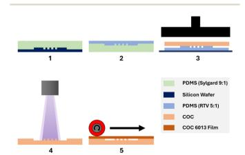
Fig. 1 Schematic summary of the COC microfabrication procedure. (1) Sylgard PDMS counter mould. (2) Replication of the microstructure of the silicon wafer on an RTV PDMS membrane. (3) Hot pressing of COC to impart microstructure. (4) Deposition of an organosilicon layer using TEOS as a precursor in the plasma process. A mask can be positioned over the COC to limit the treatment to precise zones. (5) Closing of the microfluidic
