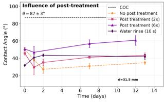
Fig. 4 Influence of post-treatments on the time variation of contact angles following silica-like surface deposition. Air plasma pre-treatment and 4 passes of the PECVD process were applied to all samples. Three conditions of plasma post-treatment are shown: 2 passes (■), 6 passes (▲), or rinsing with water for 10 s right after the deposition (\*). The torch-tosurface distance is of d = 31.5 mm for all experiments.
