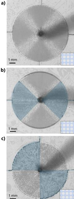
Fig. 9 Injection of a water-in-oil emulsion in a COC micromodel of variable wettability: uniformly hydrophobic ((a), contact angle 87°) and mixed (b)-(c). Hydrophilic zones (contact angle 40°) have been colored in blue in the images. Grey-level within the micromodels indicates the concentration of dyed water droplets.
