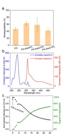
(a) The degradation of PG and PG-dopa nanoparticles in 1 U  $\alpha$ -amylase PBS solution after 3 h. (b) Fluorescence excitation and emission spectra of PG-dopa10% films. (c) PG-dopa10% coated quartz incubated in  $\alpha$ -amylase (45 U mL $^{-1}$ ) PBS solution, with fluorescence intensity monitored as a function of time. The excitation and emission wavelengths are 280 nm and 310 nm
