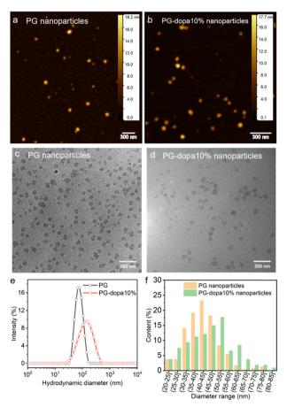
Fig. 2 (a) Dry state AFM topography image of PG nanoparticles. (b) Dry state AFM topography image of PG-dopa nanoparticles. (c) TEM image of PG nanoparticles. (d) TEM image of PG-dopa10% nanoparticles. (e) DLS hydrodynamic diameter populations of PG and PG-dopa nanoparticles. (f) Calculated diameter range populations of PG and PG-dopa10% nanoparticles from Fig. 3(c) and (d).
