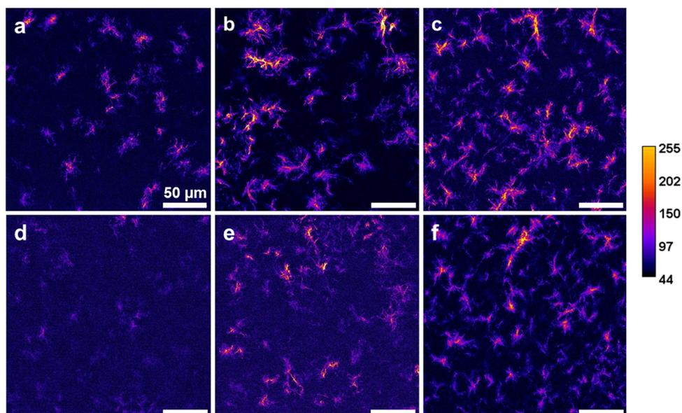
Fig. 3 SHG microscopy images of hydrogels at (a) 10%, (b) 20% and (c) 30% using the vapour process and (d) 10%, (e) 20% and (f) 30% using the wet process. Scale bar: 50  $\mu\text{m}$ . The lateral bar scales the SHG signal intensity.
