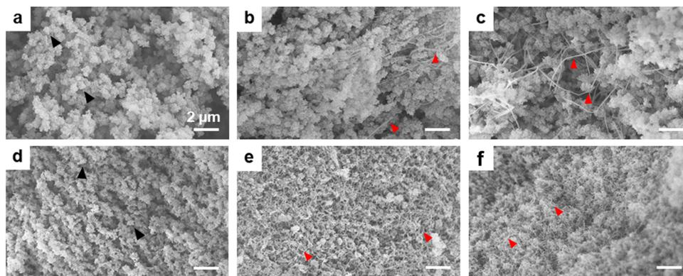
Fig. 5 SEM micrographs of (a) chitosan, (b) 10%, (c) 30% hydrogels using the vapour process and (d) chitosan, (e) 10%, (f) 30% hydrogels using the wet process. Scale bar: 2  $\mu\text{m}$ . Red arrows indicate collagen fibrils. Black arrows indicate chitosan nanoaggregates.
