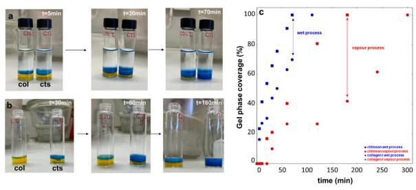
Fig. 7 Study of the kinetics of gelation. Visual evolution in the presence of bromothymol blue of collagen (col) and chitosan (cts) solutions at  $25 \text{ mg m} \text{L}^{-1}$ (a) mixed with ammonia and (b) under ammonia vapours. (c) Evolution of sol-gel coverage for both solutions and both gelation routes.
