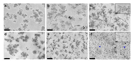
Fig. 6 TEM micrographs of (a) chitosan, (b) 10%, (c) 30% hydrogels using the vapour process and (d) chitosan, (e) 10%, and (f) 30% hydrogels using the wet process. Scale bar: 1 μm (insets, scale bar 500 nm). White arrows highlight chitosan-collagen contact points and blue arrows indicate collagen fibrils.
