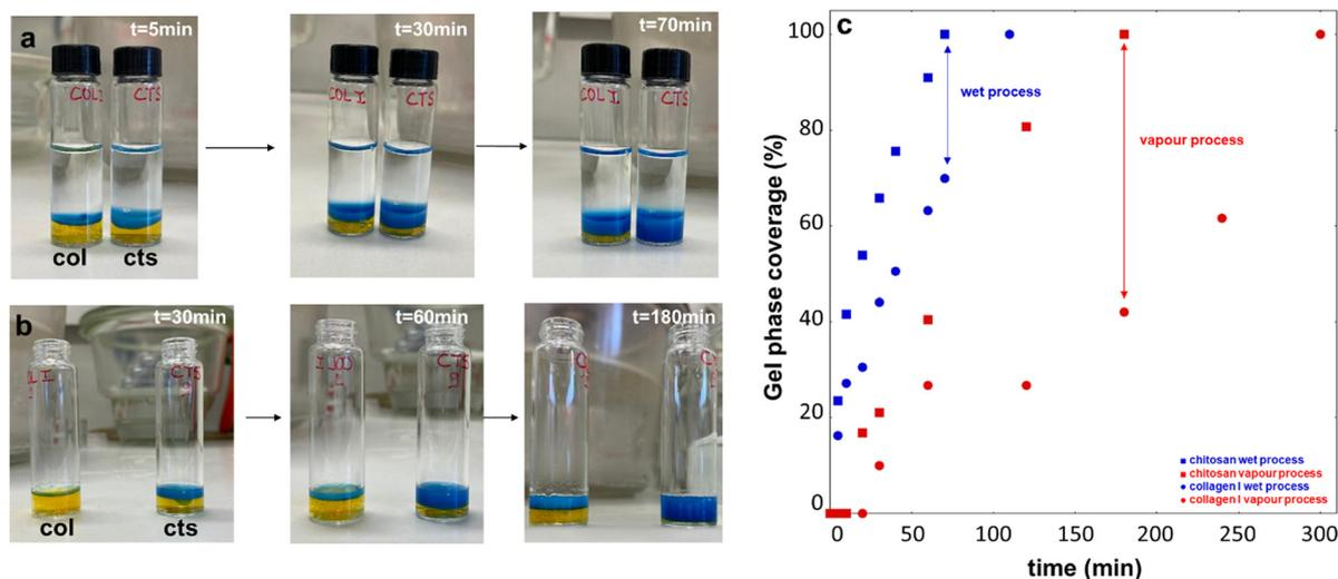
Fig. 7 Study of the kinetics of gelation. Visual evolution in the presence of bromothymol blue of collagen (col) and chitosan (cts) solutions at  $25 \text{ mg mL}^{-1}$  (a) mixed with ammonia and (b) under ammonia vapours. (c) Evolution of sol-gel coverage for both solutions and both gelation routes.
