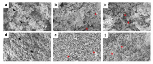
Fig. 5 SEM micrographs of (a) chitosan, (b) 10%, (c) 30% hydrogels using the vapour process and (d) chitosan, (e) 10%, (f) 30% hydrogels using the wet process. Scale bar: 2 µm. Red arrows indicate collagen fibrils. Black arrows indicate chitosan nanoaggregates.
