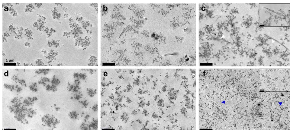
Fig. 6 TEM micrographs of (a) chitosan, (b) 10%, (c) 30% hydrogels using the vapour process and (d) chitosan, (e) 10%, and (f) 30% hydrogels using the wet process. Scale bar: 1  $\mu\text{m}$  (insets, scale bar 500 nm). White arrows highlight chitosan-collagen contact points and blue arrows indicate collagen fibrils.
