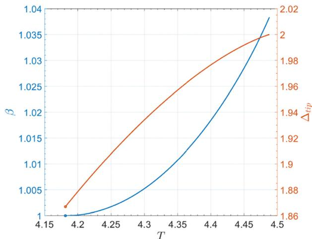
Fig. 7 Normalized crack length  $\beta$  (blue line) and  $\Delta_{\text{tip}}$  (red line) versus normalized time  $T$  for  $\alpha = 1.1 < \alpha^* = 1.7071$ . Simulations used  $\beta_0 = 1$ ,  $\eta_{\text{max}} = 1$ , and  $\phi_{\text{max}} = 2$ . Note  $\alpha = 1.1$ , slightly above  $\eta_{\text{max}} = 1$ .
