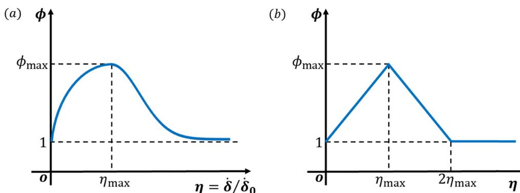
Fig. 3 Schematic of  $\phi = \delta_c/\delta_0$  as a function of  $\eta = \dot{\delta}/\dot{\delta}_0$ . (a) Shows a general function of  $\phi(\eta)$  which starts at  $\phi(\eta = 0) = 1$ , monotonically increases to  $\phi_{\max}$  at  $\eta = \eta_{\max}$  and then monotonically decreases to 1 as  $\eta \rightarrow \infty$ . (b) Is the piecewise-linear function we use in this paper for analytical analysis in the section called fracture initiation.
