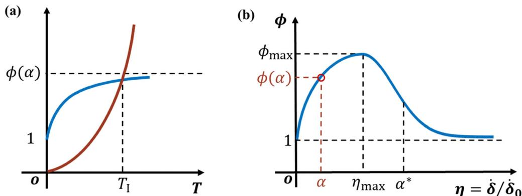
Fig. 9 Schematic illustration of case 1 where  $\alpha \leq \eta_{\max}$  for fracture initiation. (a) Blue curve is the RHS of (22), i.e.,  $\phi$  while red curve is the LHS, i.e.,  $\Delta_{\text{tip}}$ , the intersection gives the initiation time. (b) Schematic plot of the shear response function  $\phi$  showing relation between  $\alpha$ ,  $\eta_{\max}$  and  $\alpha^*$ . Plots not to scale.
