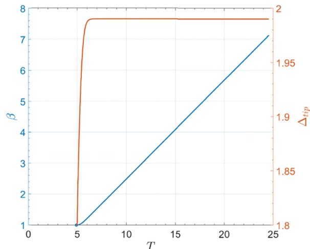
Fig. 6 Normalized crack length  $\beta$  (blue line) and  $\Delta_{\text{tip}}$  (red line) versus normalized time  $T$  for  $\alpha = 0.9 < \alpha^* = 1.7071$ . Simulations used  $\beta_0 = 1$ ,  $\eta_{\text{max}} = 1$ , and  $\phi_{\text{max}} = 2$ . Note  $\alpha = 0.9$ , slightly below  $\eta_{\text{max}} = 1$ .
