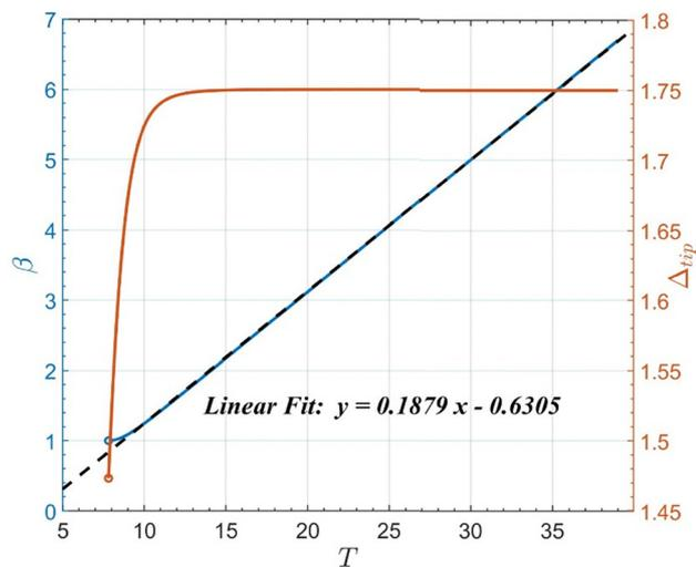
Fig. 5 Normalized crack length  $\beta$  (blue line) and  $\Delta_{\text{tip}}$  (red line) versus normalized time  $T$  for  $\alpha = 0.5 < \alpha^* = 1.7071$ . Simulations used  $\beta_0 = 1$ ,  $\eta_{\text{max}} = 1$ , and  $\phi_{\text{max}} = 2$ . The black dashed line is the linear fit of  $\beta(T)$  with slope 0.1879.
