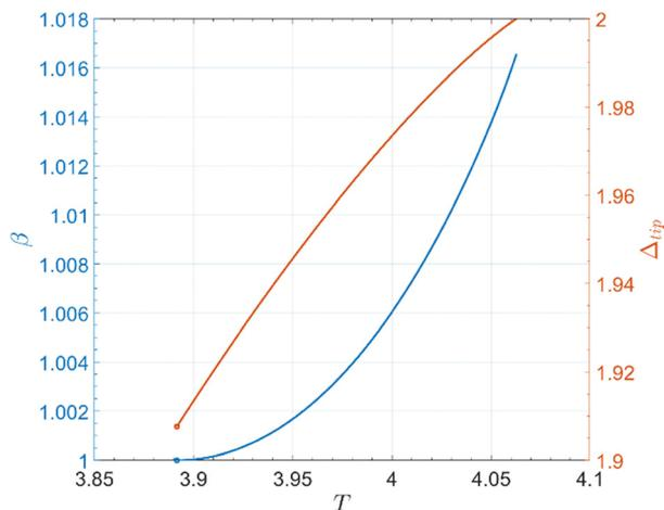
Fig. 8 Normalized crack length  $\beta$  (blue line) and  $\Delta_{tip}$  (red line) versus normalized time  $T$  for  $\alpha = 1.2 < \alpha^* = 1.7071$ . Simulations used  $\beta_0 = 1$ ,  $\eta_{max} = 1$ ,  $\phi_{max} = 2$ .
