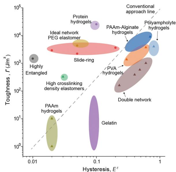
Fig. 6 Ashby plot of toughness ( $\Gamma$ ) and hysteresis based on network design. The black dashed line represents the conventional relationship between toughness and hysteresis in soft materials. Advanced network designs deviate from this conventional relationship.
