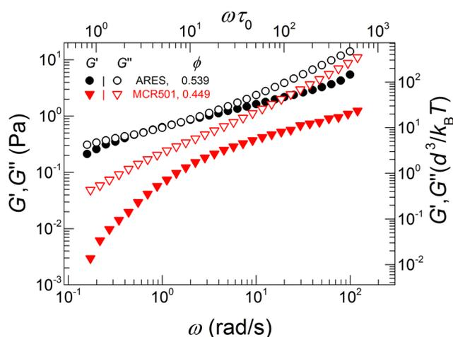
Fig. 8 Dynamic frequency sweeps of two less concentrated samples with  $\phi = 0.539$  and  $\phi = 0.449$  exhibiting moduli crossover and  $\tan \delta$  minimum, respectively. Particles are PMMA hard spheres of radius  $R_{\text{h}}$  of 264 nm dispersed in squalene at  $T = 23$  °C. Measurements were performed using the MCR 501 and ARES rheometers.
