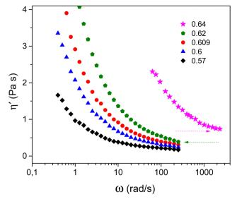
Fig. 10 The in-phase with the strain rate dynamic viscosity limiting behavior of hard spheres,  $R_h$  = 264 nm, dispersed in squalene at T = 23 °C. The legend indicates the experimentally estimated volume fraction. Data for  $\phi$  = 0.64 (magenta symbols) are measured with a PZR of up to 3000 rad s<sup>-1</sup>. Horizontal arrows indicate high frequency viscosity determination for the two highest volume fractions shown.
