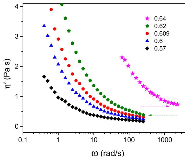
**Fig. 10** The in-phase with the strain rate dynamic viscosity limiting behavior of hard spheres,  $R_p = 264$  nm, dispersed in squalene at  $T = 23$  °C. The legend indicates the experimentally estimated volume fraction. Data for  $\phi = 0.64$  (magenta symbols) are measured with a PZR of up to  $3000$   $\text{rad s}^{-1}$ . Horizontal arrows indicate high frequency viscosity determination for the two highest volume fractions shown.
