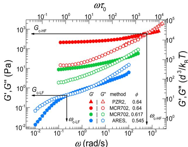
Fig. 3 Dynamic frequency sweeps of concentrated ( $\phi = 0.64, 0.617$  and  $0.545$ ) hard spheres ( $R_h = 264 \text{ nm}$ ) dispersed in squalene at  $T = 23 \text{ }^\circ\text{C}$ . Measurements were performed using various commercial rotational rheometers such as MCR 702, ARES, and our in-lab developed PZR as indicated. Vertical and horizontal arrows point to the dynamic moduli crossover frequency,  $\omega_c$ , and modulus (magnitude),  $G_c$ , respectively.
