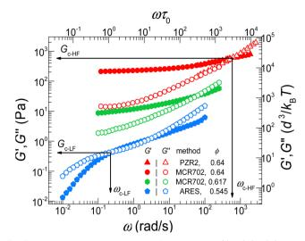
Fig. 3 Dynamic frequency sweeps of concentrated ( $\phi$  = 0.64, 0.617 and 0.545) hard spheres ( $R_h$  = 264 nm) dispersed in squalene at T = 23 °C. Measurements were performed using various commercial rotational rheometers such as MCR 702, ARES, and our in-lab developed PZR as indicated. Vertical and horizontal arrows point to the dynamic moduli crossover frequency,  $\omega_c$ , and modulus (magnitude),  $G_c$ , respectively.
