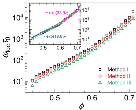
Fig. 6 Volume fraction dependence of the dimensionless localization frequency,  $\omega_{\text{loc}}\tau_0 \equiv \tau_0/t_{\text{loc}}$ , based on the 3 theoretical methods I, II and III described in the text. (inset) Same display as in the main frame but with red and green data vertically shifts up by multipliers of 1.25 and 1.7, respectively.
