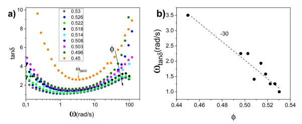
Fig. 11 LVE data for samples with  $\phi < \phi_{ons} = 0.54$ , where no G', G'' crossover is exhibited. (a) Loss angle tangent dependence on the angular frequency; different  $\varphi$  values, as indicated, increase as shown by a solid black arrow; a vertical arrow indicates the minimum of  $\tan \delta$  (for  $\varphi = 0.45$ ) where  $\omega_{\tan \delta}$  is determined. (b) Frequency of the minimum in  $\tan \delta$  plotted as a function of  $\phi$ . The dashed line is the best data fit.
