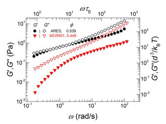
Fig. 8 Dynamic frequency sweeps of two less concentrated samples with  $\phi$  = 0.539 and  $\phi$  = 0.449 exhibiting moduli crossover and  $\tan \delta$  minimum, respectively. Particles are PMMA hard spheres of radius R<sub>h</sub> of 264 nm dispersed in squalene at T = 23 °C. Measurements were performed using the MCR 501 and ARES rheometers
