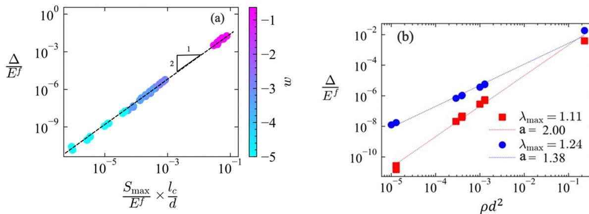
Fig. 7 (a) Dissipation per loading–unloading cycle and per unit volume of the network during stress control loading of non-affine networks with a broad range of  $w$  and with  $\bar{S}_i^f = 0.01$  and  $\bar{E}_p^f = 0.5$ , function of  $d/l_c$  and the stress at unloading,  $S_{\max}$ . (b) Dissipation per loading–unloading cycle and per unit volume of the network during strain control loading for a range of  $d/l_c$  and two maximum stretches,  $\lambda_{\max} = 1.11$  and  $1.25$ .
