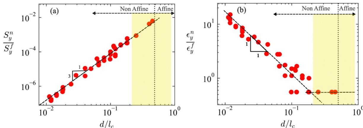
Fig. 2 (a) Network yield stress normalized by the yield stress of fibers,  $S_y^n/S_y^f$ , vs.  $d/l_c$ , and (b) network yield strain normalized by the yield strain of fibers,  $\epsilon_y^n/\epsilon_y^f$ , vs.  $d/l_c$ . The non-affine to affine transition is shown by the vertical yellow band and  $w_0$  is marked by the dotted line. Each data point corresponds to a single realization. A total of 8 network realizations have been used to produce these plots.
