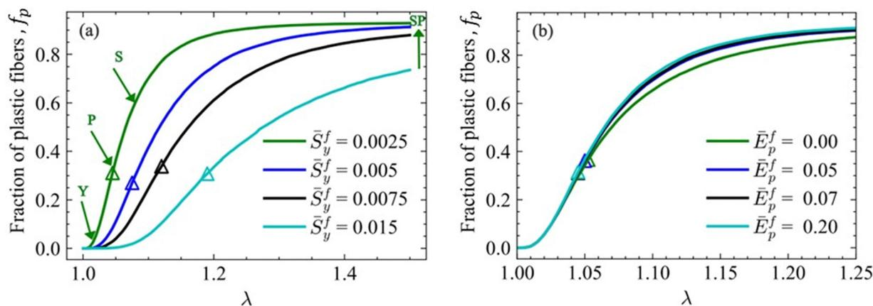
Fig. 4 Fraction of plastic fibers vs. stretch for all cases shown in Fig. 3, *i.e.* for networks with  $w = -3.54$  and (a) same  $\bar{E}_p^f = 0.07$  and different fiber yield stresses, and (b) same  $\bar{S}_y^f = 0.0025$  and different fiber plastic stiffening rates,  $\bar{E}_p^f$ . Open triangles show plastic percolation.
