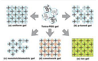
Fig. 13 Schematics of the derivatives of tetra-PEG gels: (a) uniform gels, (b) p-tuned gels, (c) nonstoichiometric gels, (d) conetworks, and (e) ion gels. Black and grey lines show a set of NHS-terminated tetra-PEG and amine-terminated tetra-PEG macromers, or a set of maleimideterminated and thiol-terminated tetra-PEG macromers. Red lines denote environment-sensitive macromers, such as thermosensitive macromers, The yellow box shows an ionic liquid environment instead of an aqueous
