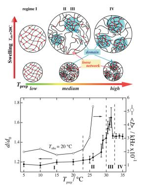
Fig. 9 (Top) Gel inhomogeneity model for PNIPAM gels prepared at different temperatures  $T_{\text{prep}}$  and observed at  $T_{\text{obs}}$  = 20 °C. (Bottom) Linear swelling ratio  $d/d_0$  vs.  $T_{\rm prep}$  (left; filled circles) and light scattering intensity  $\langle I \rangle_{\rm E}$  vs.  $T_{\rm prep}$  (right; open circles). 60 (Modified from parts of Fig. 4 in ref. 49.)
