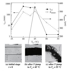
**Fig. 8** Shrinking kinetics of PNIPAM gels with T-jumps to different temperatures,  $T_{\rm d}$ . Set (Upper)  $t_{1/2}$  (left) and  $d_{\rm opaque}$  (right) vs.  $T_{\rm d}$ . (Lower) Optical photographs of the gel (a) in the initial state, and after T-jumping to (b)  $T_{\rm d}$  = 45 °C and (c) to  $T_{\rm d}$  = 55 °C. (Modified from parts of Fig. 3 in ref. 49.)
