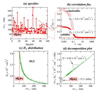
Fig. 10 DLS decomposition plot. (a) Speckles, (b) correlation functions, (c)  $D_{\rm A}$  distribution, and (d) decomposition plot. (Reprinted with permission from ref. 71. Copyright 2006 Chemical Society of Japan.)
