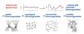
Fig. 11 Various types of inhomogeneities. (Upper row) Schematics of concentration fluctuations: (left) polymer solutions and (right) polymer gels where frozen inhomogeneities (blue) are introduced by cross-linking, superimposed onto thermal fluctuations (red). (Lower row; from left to right) (a) Spatial, (b) topological, (c) connectivity, and (d) mobility inhomogeneities.
