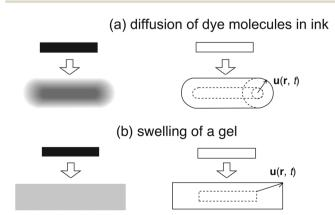
Fig. 4 Comparison of (a) diffusion of ink dye molecules on a wet filter paper and (b) swelling of a piece of gel.  $\mathbf{u}(\mathbf{r}, t)$  is the displacement vector.
