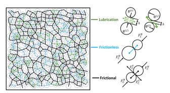
Contact network inferring all forces. Snapshot of the contact network for  $\phi = 0.76$  and  $\sigma/\sigma_0 = 1$ . Green, blue, and black lines depict lubrication, frictionless, and frictional interactions, respectively
