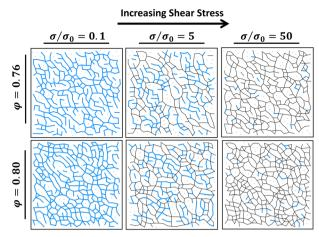
Fig. 4 Development of frictional contacts with increasing shear stress Snapshots of the contact network for both frictionless (normal force below the critical threshold  $F_0$ ) shown as blue lines and frictional contacts (normal force above the critical threshold  $F_0$ ) as black lines. Snapshots corresponding to simulations with  $\sigma/\sigma_0$  = 0.1, 5, 10, and 50 (from left to right) are presented for  $\phi = 0.76$  (top) and  $\phi = 0.8$  (bottom).
