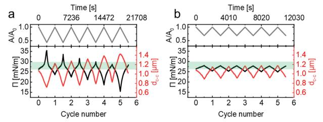
Fig. 5 Repeated compression/expansion cycles (each at 3 mm min $^{-1}$ ). Surface pressure  $\Pi$  and interparticle distance  $d_{c-c}$  as a function of cycle number and the normalized area  $A/A_0$  as a function of time as a reference are shown. (a) Cycles compressed beyond region II and (b) with adjusted parameters to not exceed region II are presented. The green-colored area marks region II.
